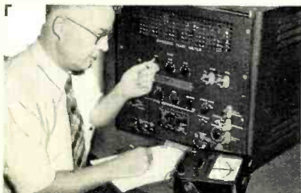
Dynamic Fluxmeter, developed by Bell Laboratories, indicates flux build-up in intervals of 25 millionths of a second. Precise information like this was essential to higher speed operation.
