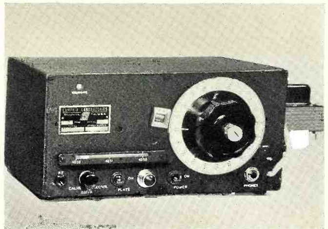
The Lampkin Type 105-B micrometer frequency meter. It is used to measure the center frequency of AM or FM transmitters.
