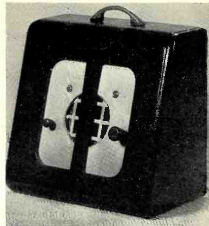
Front view of the home-built intercom. The entire unit is housed in a compact and inconspicuous cabinet. A spring-loaded switch is actuated when unit is used to transmit and released during reception.
