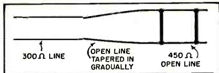
Fig. 20. How to connect a 450-ohm line to a 300-ohm line without having a mismatch.
