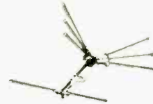
3. JeTenna elements lock into position effecting 35 forward inception angle and 40 dipole angulation for greater signal pickup. Reflectors snap into place for quick tightening by wing nuts.
