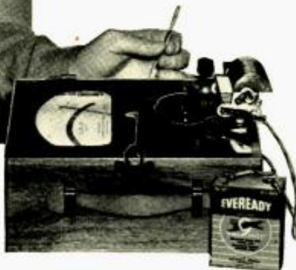
Duplicating one of the principles of the new generator can be done by using a steatite condenser, 1000 volt electrostatic meter, and a 67½ volt "B" battery.
