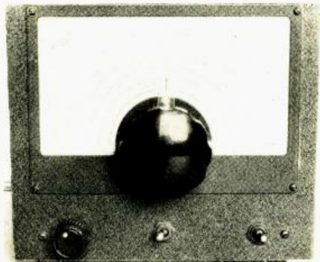
Front panel view. Controls include the variable condenser across mixer coil, standby switch, and b.f.o. "on-off" switch. Main tuning is accomplished by large vernier dial in the center.
