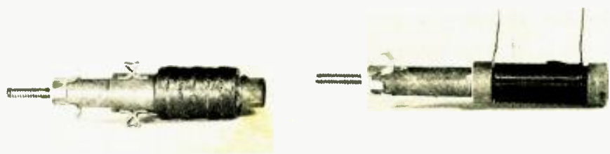
Fig. 3. The RAM 201R3 linearity coil (left) and 201R1 width coil (right).
