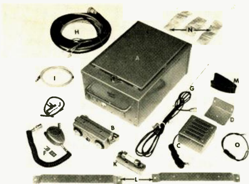
Components comprising a single mobile radio unit. (A) The transmitter, receiver, and power supply. (B) Control unit for dash mounting—includes pilot lights, volume control, squelch control, and channel selector switch. (C) Loudspeaker. (D) Mounting bracket for speaker. (E) Microphone. (F) Microphone mounting clip. (G) Quarter-wave whip antenna for car-top mounting with flexible coaxial cable. (H) Multi-conductor cable to interconnect control unit and radio unit. (I) Wire for connecting hot side of battery to fuse. (J) Interference filter. (K) Fuse and mount. (L) Mounting brackets. (M) Loom for protecting cable from wear. (N) Screws and miscellaneous hardware. (O) Metering plug and cable for testing the operation of the entire unit.
