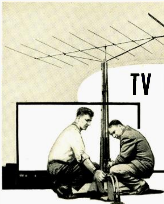
The author, with Hazeltine engineer, points to shielded down-lead connecting antenna to lab instruments.
