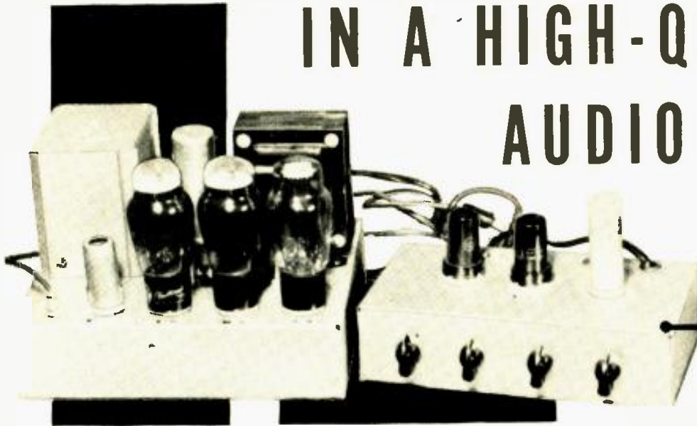
Fig. 1. Over-all view of the power amplifier and control unit which was designed around the new miniature, 9-pin 6U8 combination triode and pentode.
