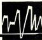
Fig. 1. A type of interference due to slope detection. This circuit fault was fairly common in the early intercarrier video sets.
