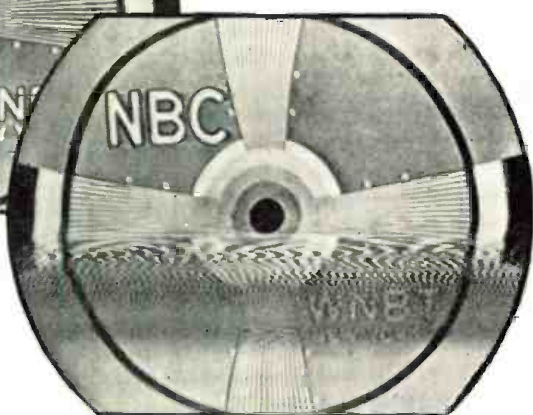
Fig. 8. This familiar type of interference is caused by diathermy equipment operated in vicinity.
