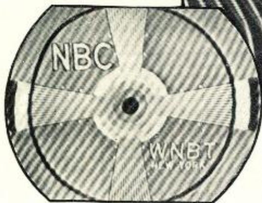
Fig. 3. This is how r.f. interference appears on screen. Oblique lines and haziness are present.
