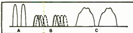
Fig. 2. (A) Initial pulses generated by musical instrument or other source. (B) Initial pulses and delayed pulses produced by wall reflections. (C) Combination of initial and reflected pulses showing a tone which contains much greater average energy and low-frequency content than (A) or (B).
