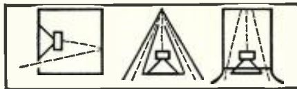
Fig. 7. Several known types of speaker baffles in which back radiation is used and influences reproduction of pulses. The acoustic delay path is shown dotted.
