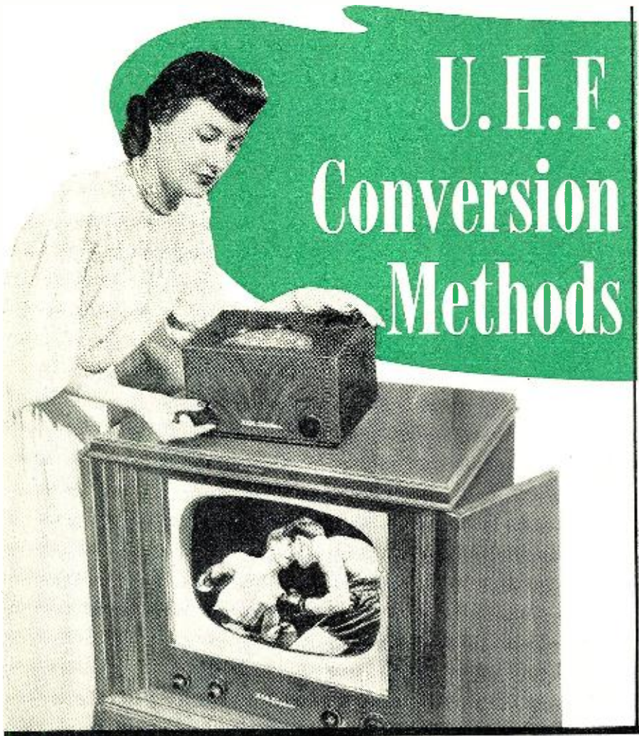
Fig. 1. RCA's ultra-high-frequency converter for use in any area having u.h.f. stations. It provides coverage of the entire u.h.f. band. The unit is housed in a compact cabinet which has two knobs—the left-hand knob has three positions ("off," v.h.f., and u.h.f.) while the right-hand knob is for tuning. This converter is designed to be used with any present-day video receiver.
