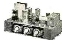
Model P-10A, 10 watt Phonograph Amplifier
