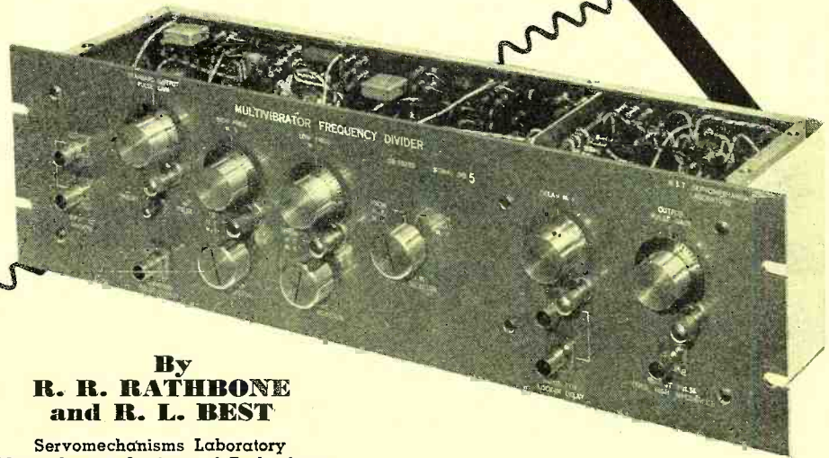
Fig. 1. Front panel view of the M.I.T. multivibrator frequency divider.
