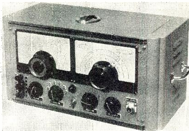
Fig. 11. Front panel view of the sweep frequency generator. The controls on the front of the panel include the marker frequency dial, band center frequency dial, phasing control, marker bandswitch, power switch, frequency deviation control, and the r.f. output control. The time base generator switch and phasing control are behind panel.
