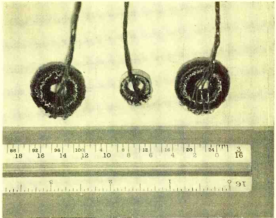
Multi-stable magnetic memory elements for storing large numbers of pulses.
