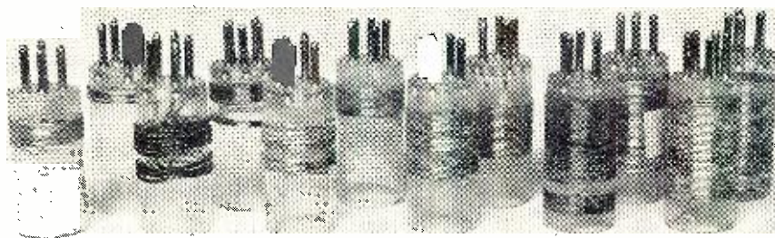
Fig. 5. Midget plug-in coils provide full coverage of the 75, 20, and 10 meter bands.
