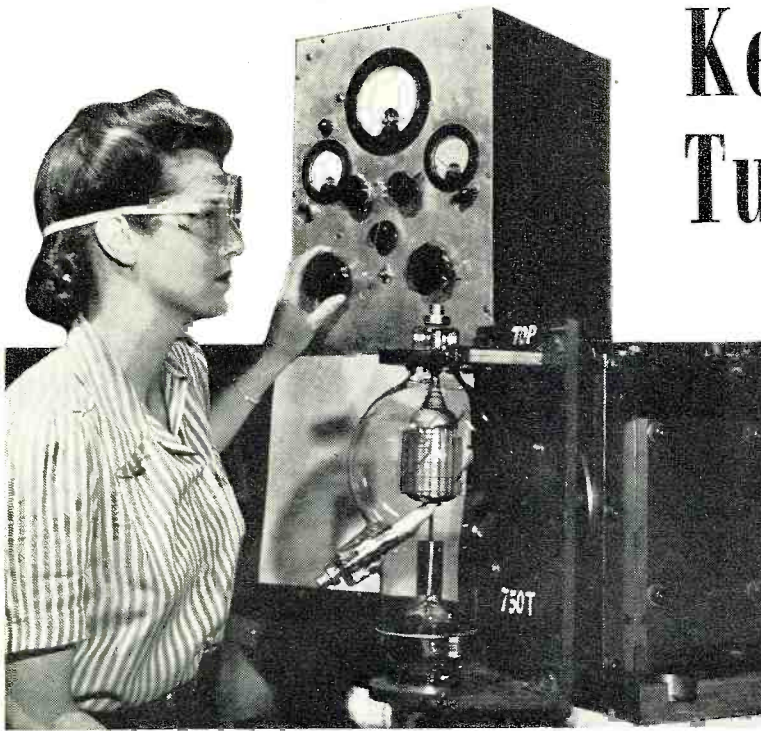
Miss Norene Evans checks an Eimac 750T to determine the amount of vibration the tube elements will withstand before shorting.
