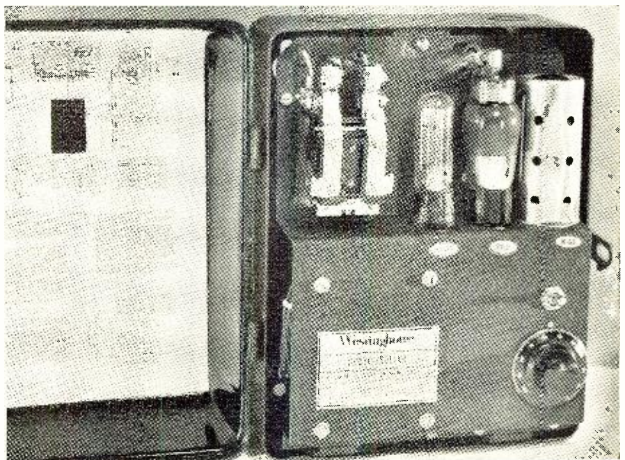
Fig. 5. Photoelectric control unit. The opened cover reveals the relay, phototube, and amplifier. In operation the light enters through the hole in cover of unit.
