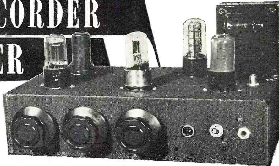
Over-all view of the auxiliary input unit used in conjunction with tape recorder.
