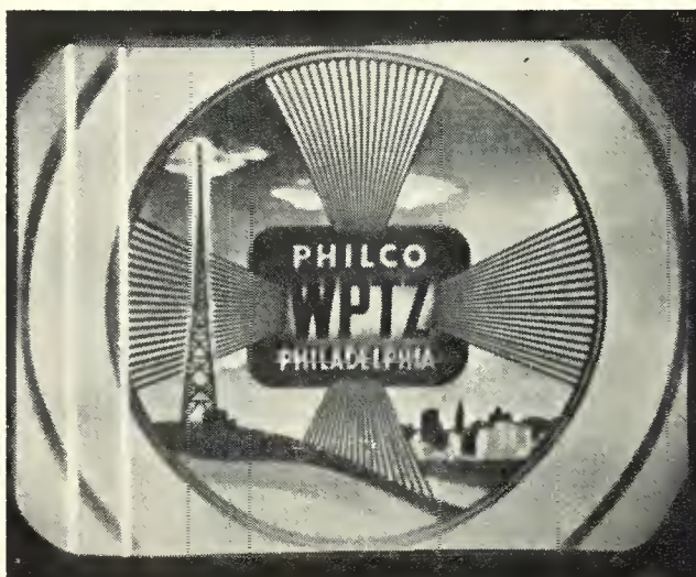
Fig. 6. Pattern showing ringing effects in horizontal output.
