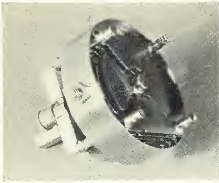
Fig. 2. Over-all view of homemade butterfly unit. The 1 3/4" diameter brass ring inductor was made by wrapping a 1/2" wide brass strip tightly around the outside of a standard butterfly tuning condenser so as to make contact with both stators. The rotors, when out of the stators, travel close to metal ring but do not make contact with it. The screw and nut holding the ends of ring together serve as "B-plus" terminal. No connection is made to the rotor plates.
