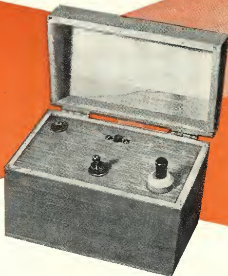
Fig. 1. Compact, self-contained micro-modulation system, housed in a small file box. Battery-type tubes are used.
