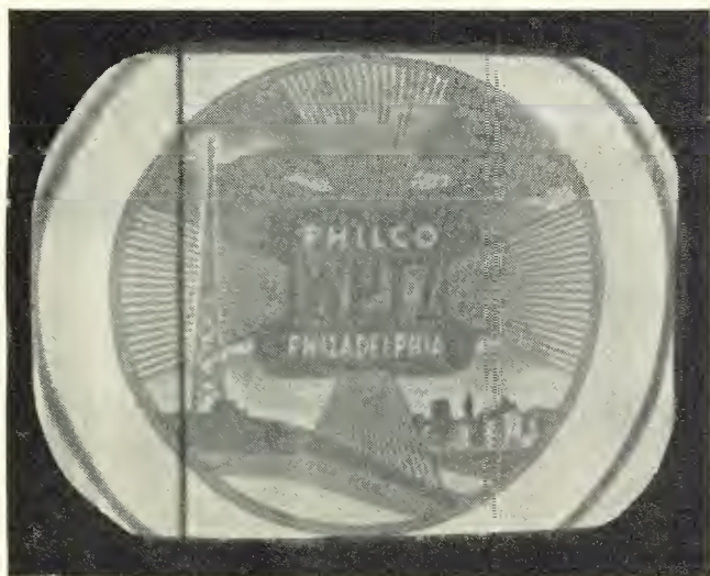
Fig. 5. Interference (black line) from Barkhausen oscillation.
