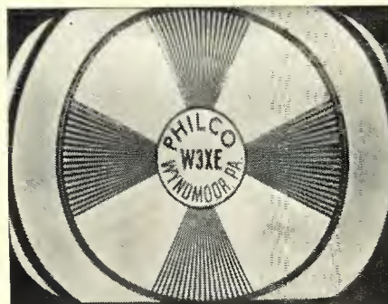
Fig. 4. Moire effect seen in the horizontal wedges indicates an imperfect interlace.
