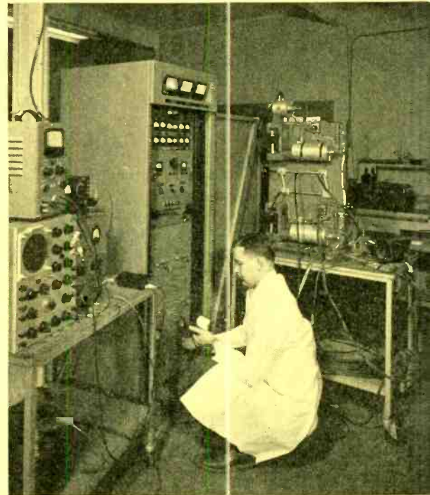
▼ Special phase-modulator tubes have been designed by the laboratory staff to incorporate the modulating jobs of several conventional u.h.f. tubes into one. The model is shown connected to the vacuum pumps during processing. Work is continuing on the development of a tube having from one to ten watts output, rather than the milliwatts output of preliminary experimental models.
