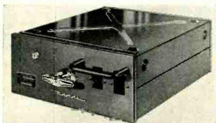
A combination receiver and 30-watt transmitter for mobile installations. Complete unit may be removed in one simple motion.
