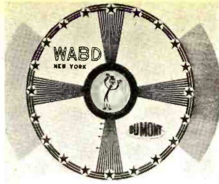
Fig. 9. Typical test pattern as received on primary channel of this installation.
