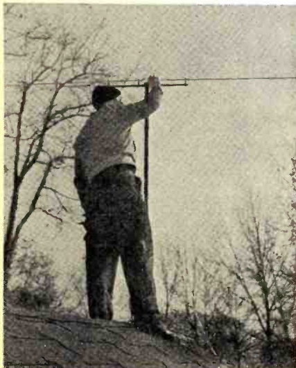
Fig. 7. The dipole is tuned by adjusting space separation between two metal rods, results being observed at TV receiver.
