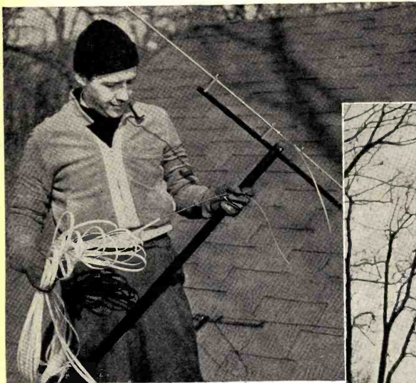
Fig. 1. The single dipole with "ribbon" lead-in and matching section is one of the simplest types of television antennas.
