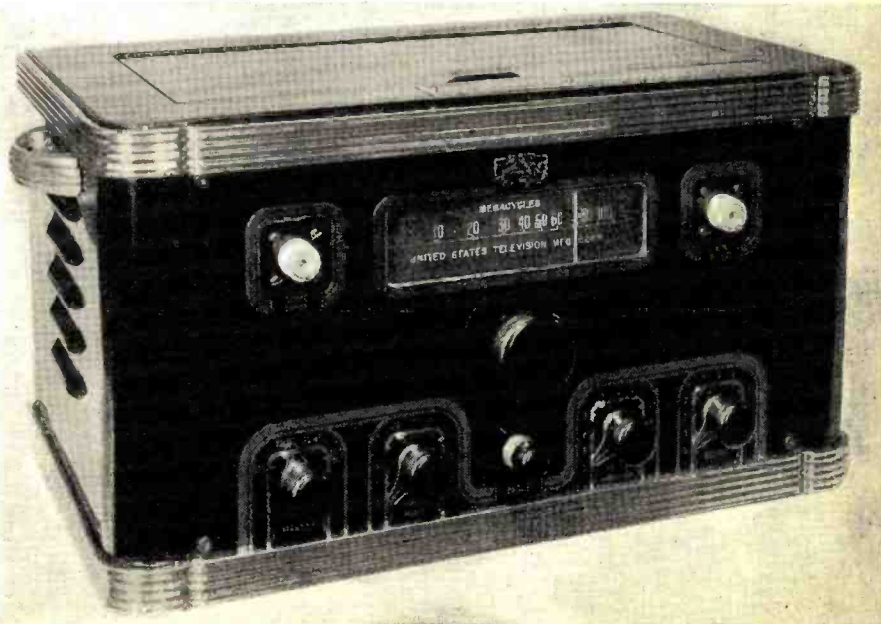
Fig. 6. High frequency signal generator built by the United States Television Mfg. Corp. The schematic diagram of this instrument is shown in Fig. 9.
