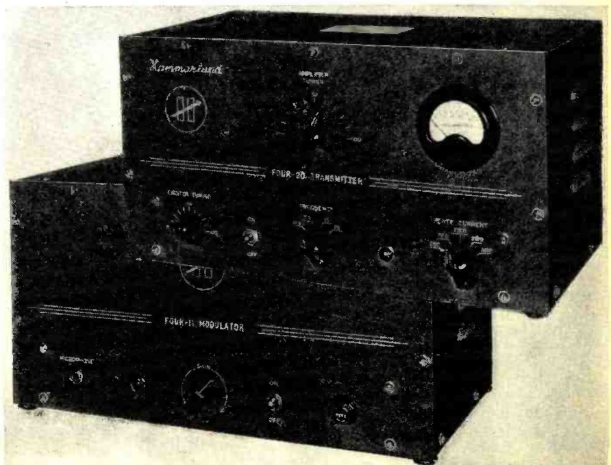
Fig. 3. The modulator unit shown is a companion to the "Four-20" transmitter.
