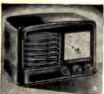
Model S-6X... a 6-tube 2-band receiver kit, equipped for either 110 or 220 volts, AC or DC covers the following ranges: 550 Kc 1600 Kc 6-16 Mc Complete and ready for assembly.
