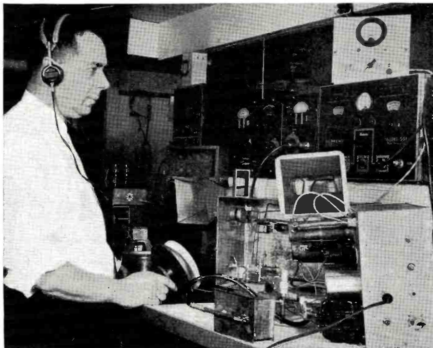
Author at work in his laboratory. Photo shows preliminary working models of microwave transmitting, receiving, modulating, and electromagnetic horn equipment.
