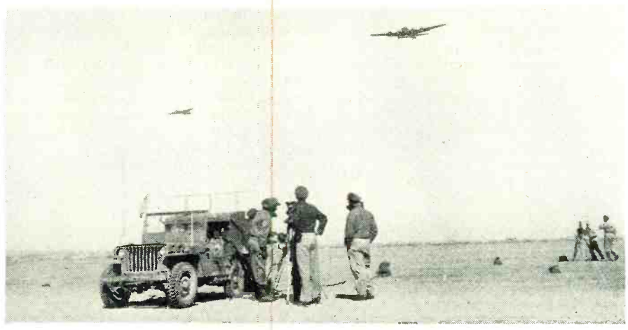
"Mother" plane hovers near her drone. In foreground a jeep control station is about to "take over" the operation of landing the drone.
