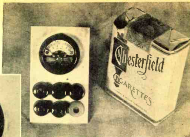
Fig. 1. Front and rear views of vest-pocket multi-range d.c. voltmeter, using a 1-inch 0-1 d.c. milliammeter. Ranges provided are 0-1, 0-10, 0-100, and 0-1000 d.c. volts and 0-1 d.c. milliamperes. Circuit schematic is given in Fig. 2. Size of the complete instrument is 2⅞" by 1-11/16" and ⅞" deep.
