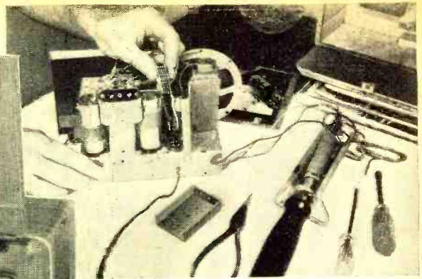
3 Two extension leads are soldered on the selenium rectifier lugs. Positive side is shown by red wire, negative by yellow or black.
