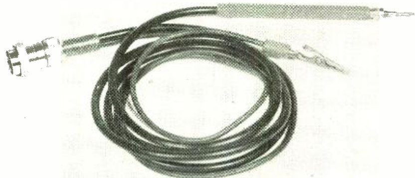
Fig. 6. D.c. test leads consisting of a shielded, single-conductor cable and ground lead.
