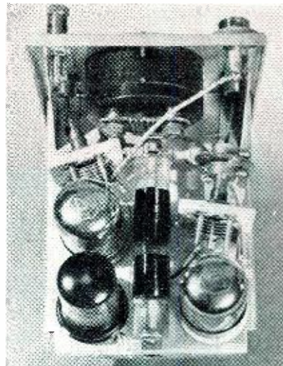
Top view of the aircraft transmitter showing compactness of assembly and proper placement of component parts.
