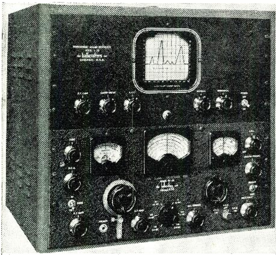
Panoramic reception shows what stations are on the air, whether phone or c.w., and their signal strengths. An instrument of this type will help keep airlines clear by reducing CQ calls to a minimum. Hallicrafters model S-35 is shown.
