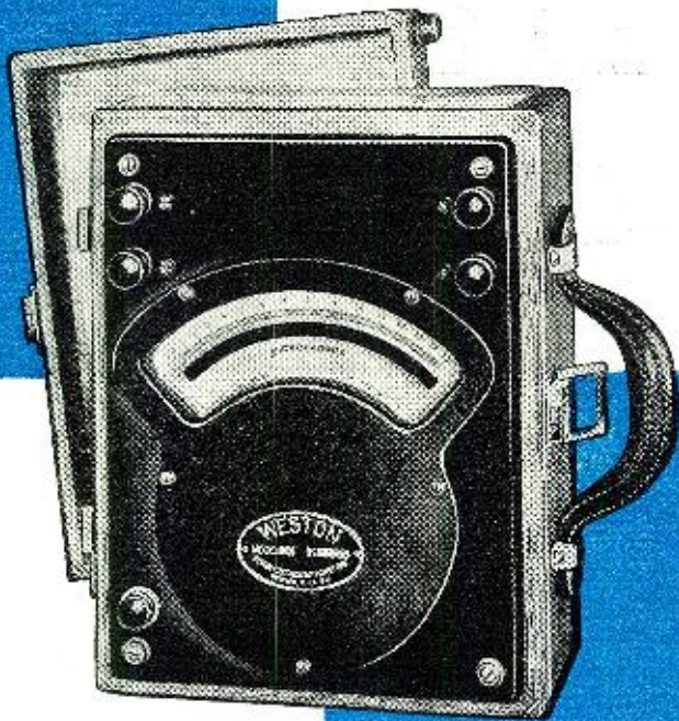
Commercially manufactured microfarad meter. This instrument is classified as a ratio type.
