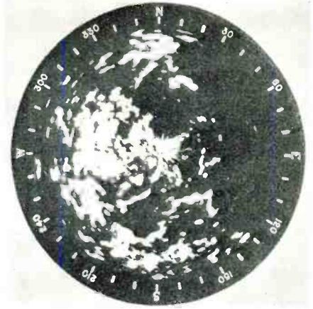
★ Closeup of a typical pattern as seen on an SG radar scope. A picture such as this affords the operator a complete picture of the territory in all directions from the ship, in spite of the fog or darkness, and may be quite readily compared with ordinary, conventional maps.
