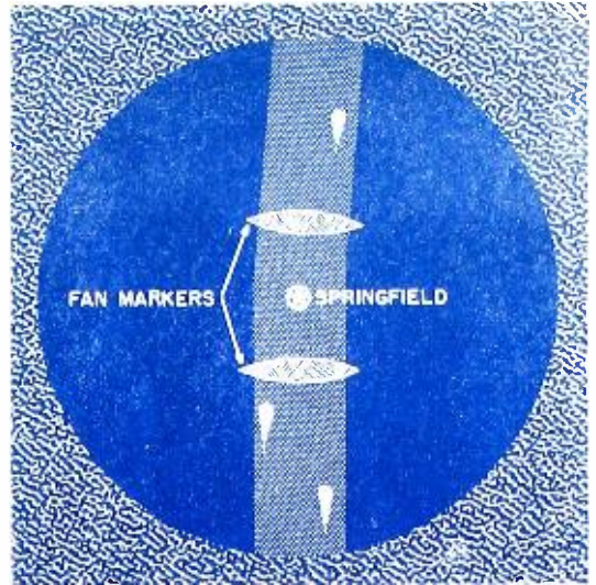
Fig. 2. A transparent map, covering an area within a radius of 50 miles, can be placed over the cathode-ray tube. Tailed light spots will indicate the location of aircraft within this area.
