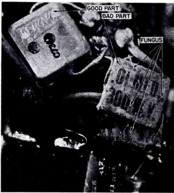
Comparison of fungus growth on properly and improperly treated components.
