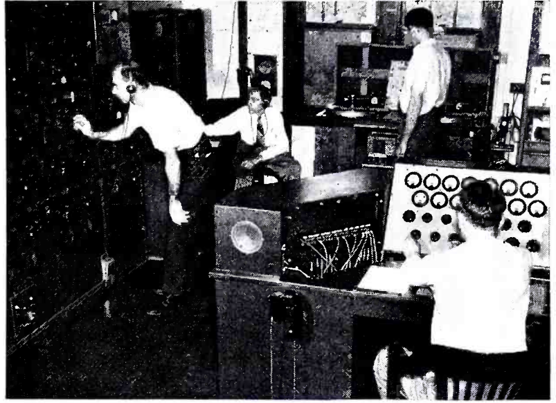
Radio transmissions are picked up by 29 SX-28 receivers and piped through the console (foreground) to the wax cylinder recorders located seven miles from this receiving station.
