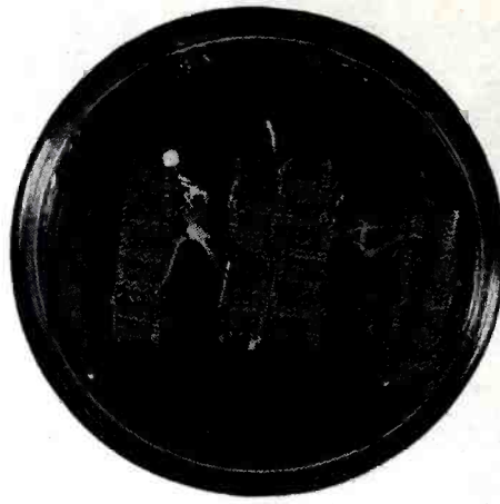
Pieces of fabric protected from fungus growth by the use of an effective fungicide.
