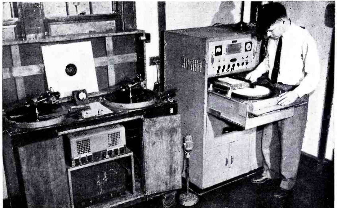
David Cooper, FBIS Supervisor, records a broadcast on a Memovox machine. Over an hour's intelligence may be recorded on each side of the flexible discs. Continuous recording is possible by using duplicate machines.
