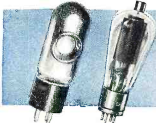
The G-E phototube and G-E thyratron are the electronic tubes used in synchronizing the operation of this packaging machine.
