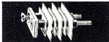
High voltage spring pile-up insulators of special heat treated Bakelite. Has minimum cold flow properties, low moisture absorption content and permits punching without cracks or checks.
