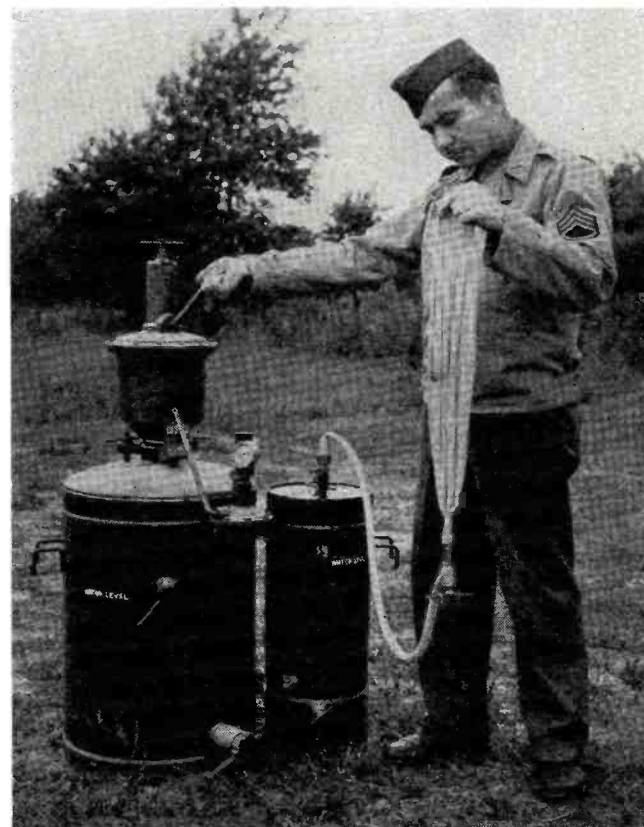
Generator, developed by the Signal Corps, is used to produce hydrogen gas for meteorological balloons, prior to their ascension.
