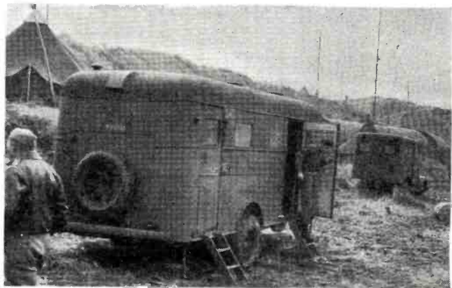
Portable radio station with antenna mast shown in right background. Trailer and power truck make up the complete unit.
