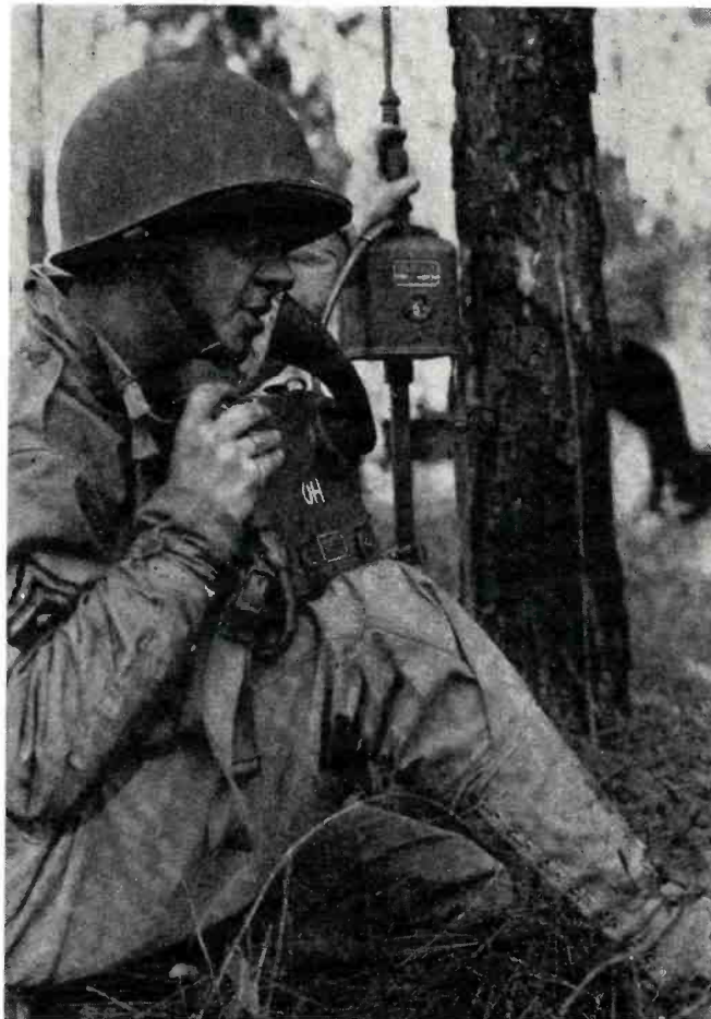
Member of Regimental Headquarters operating a late model guidon set. The r-f portion of the unit is mounted to the antenna mast.
