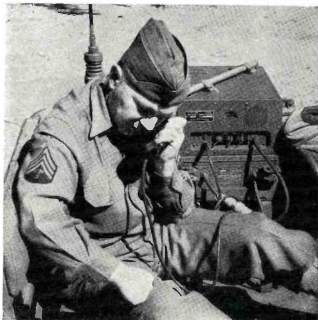
The new FM walkie-talkie. This unit has proven to be more reliable for local communications than its AM predecessor.
