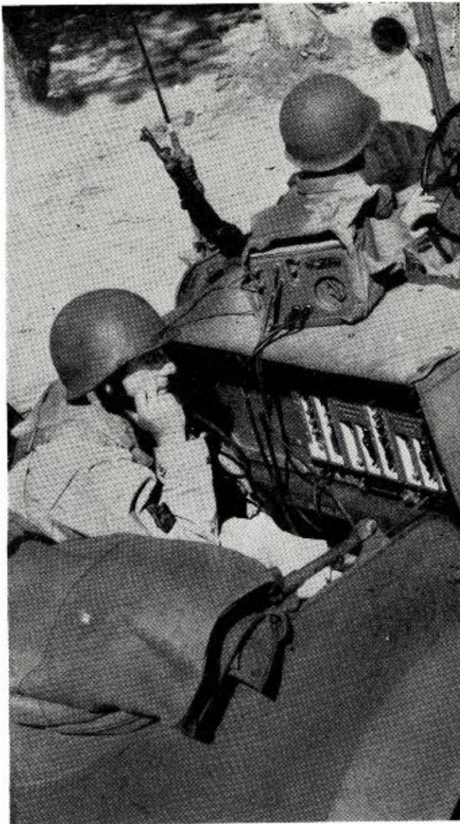
FM multi-channel transmitter and receiver used by Field Artillery.
