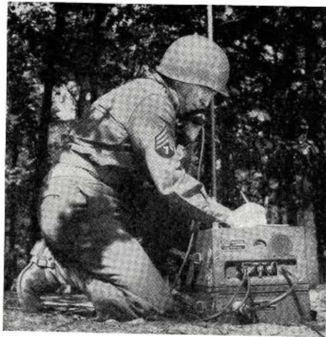
SCR-609, FM radio transmitter and receiver during field operations.
