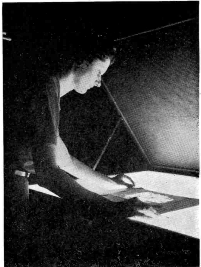
Giant contact printer used for reproducing blueprints.
