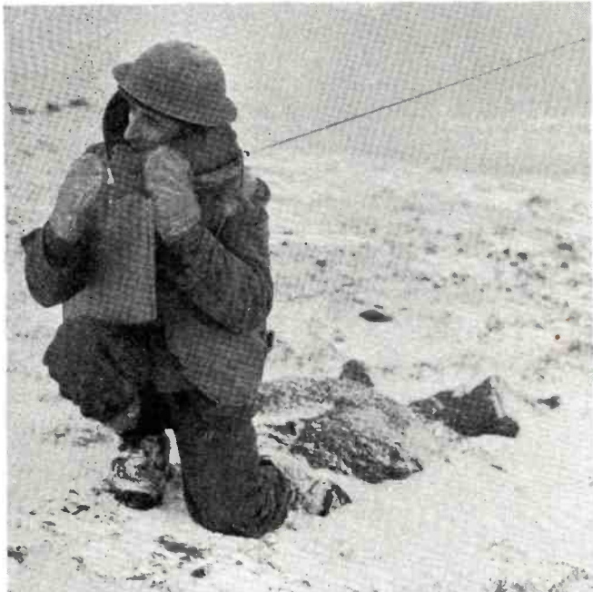
Portable field-telephone switchboard in operation. Telephone communications are a vital link between all military units.
