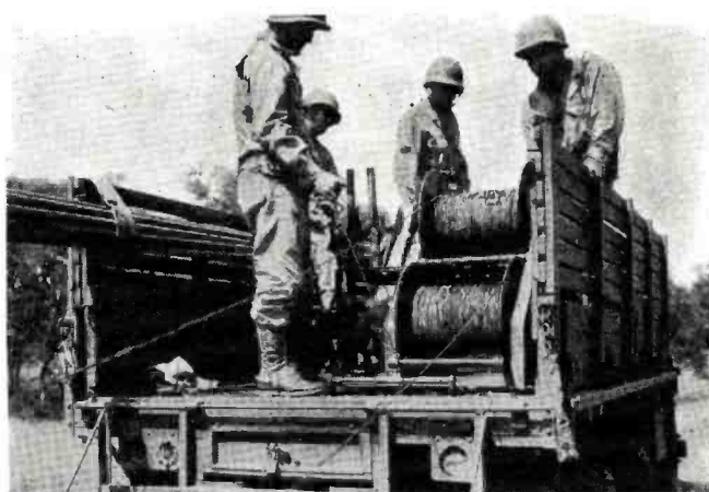
Wire laying crew and a R-L-26 on a two-and-a-half ton truck. Many miles of wire can be laid by these men in a single day.
