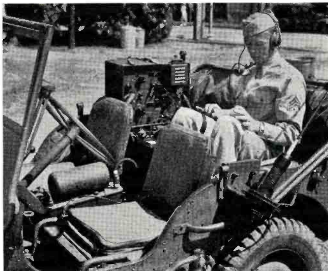
Ground portable radio set installed in jeep. Transmitter operated by telegraph key attached to the leg, or by voice telephone.
