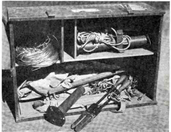
Heavy-duty soldering irons, ant. wire and supports.
