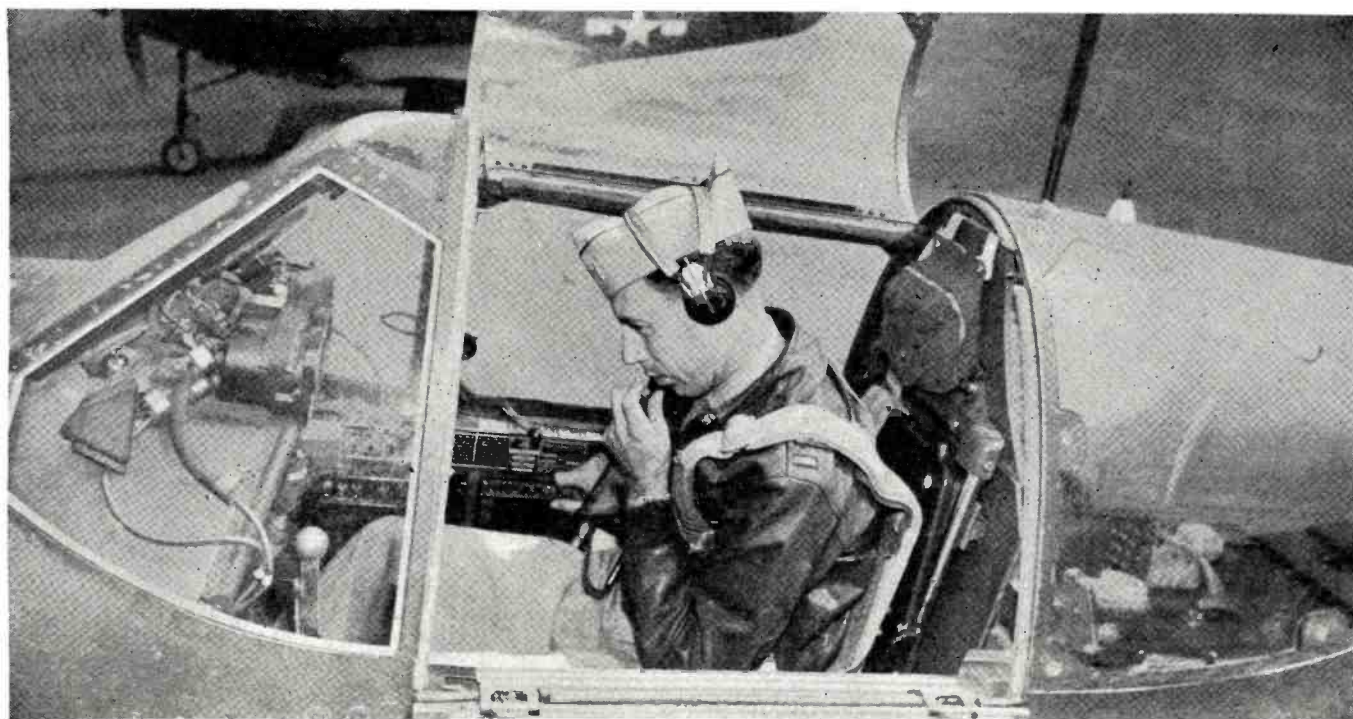
An officer of the Aircraft Laboratory testing the VHF radio equipment aboard a P-51 aircraft.
