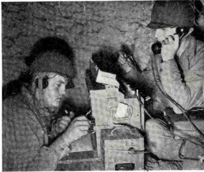
Portable field-telephone switchboard in operation. Telephone communications are a vital link between all military units.
