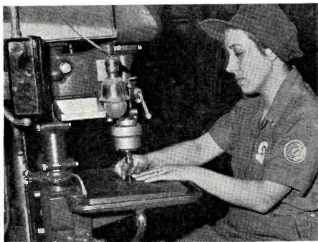
Civilian employee trained to operate high-speed tapping machine.
