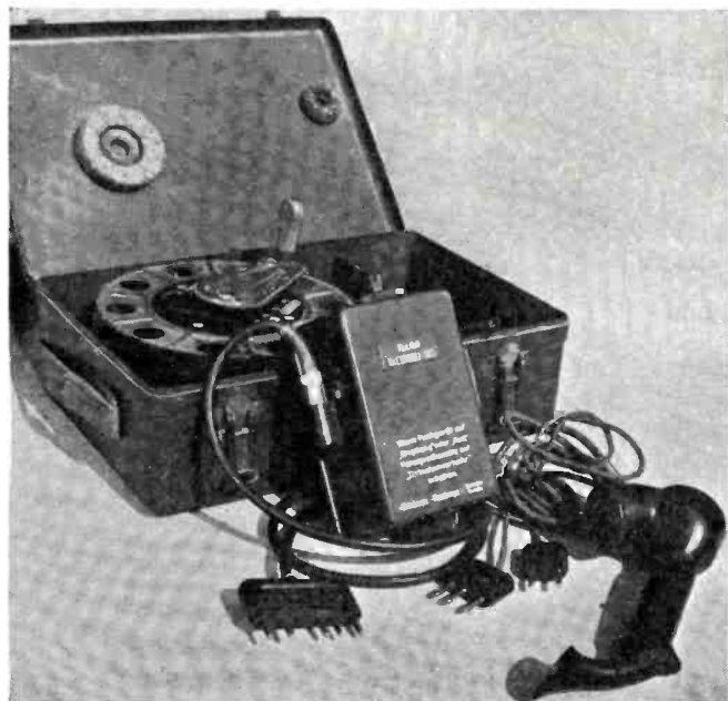
Above: Remote-control unit used in conjunction with Torn FuG, Fuheu, Fud2 and Fud1 pack sets separated to 250 yds.
