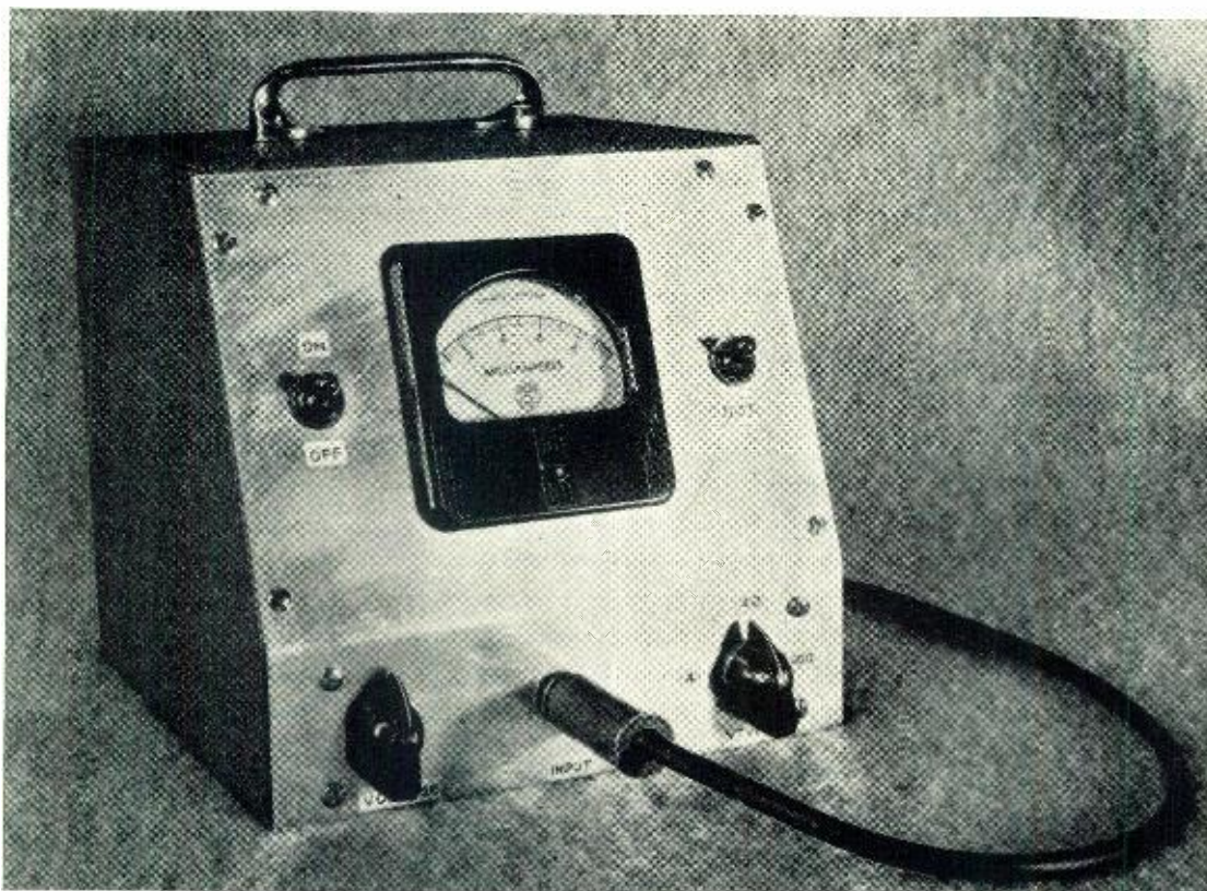
The completely assembled distortion meter, showing the front panel layout. Meter is 0-1 DCMA.
