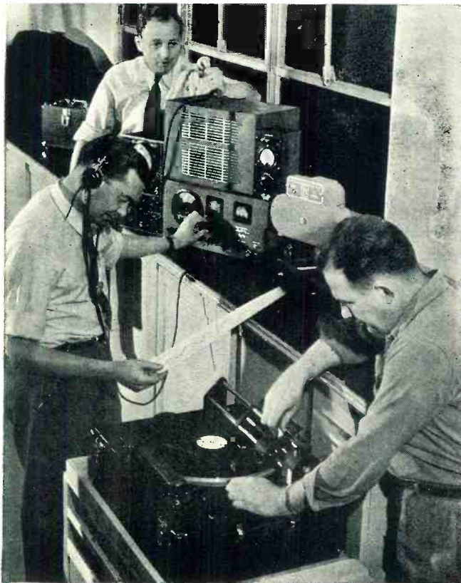
Fig. 2. Flashed to the earth by radio, the stream of reactions is picked up by the ground unit and recorded on discs.
