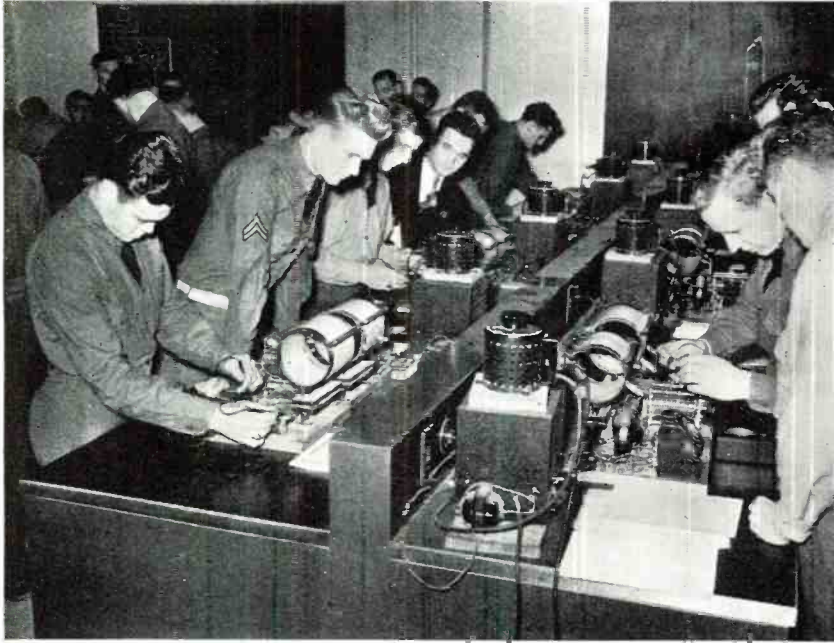
Students working with breadboard layout of Colpitts circuit. The voltage regulators help to maintain a stabilized power source.
