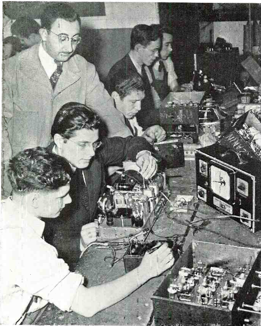
These Chelsea students are continuity testing all of the various parts used in an elaborate superhet receiver. This work is very appealing.
