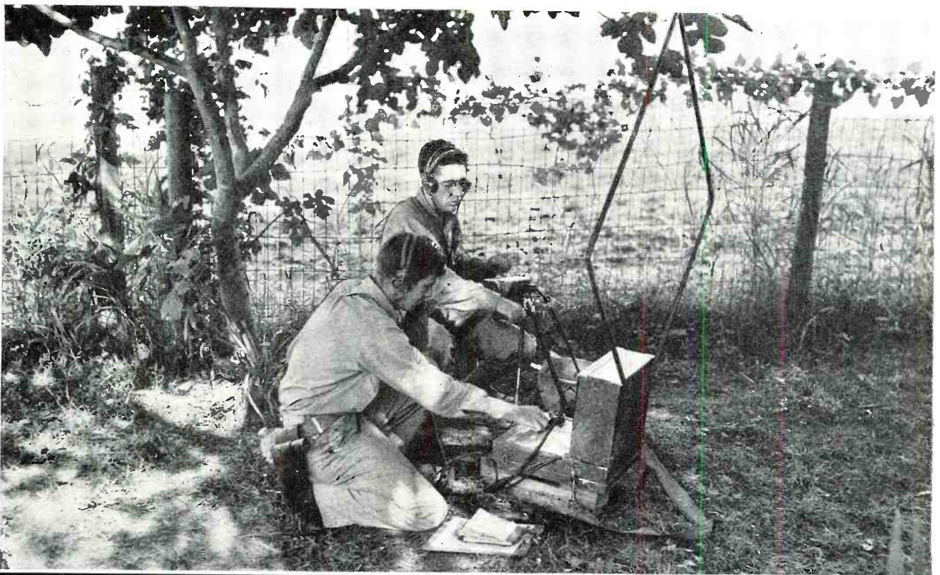
Portable transmitter-receiver gets its power from a hand operated generator. This set has loop antenna.
