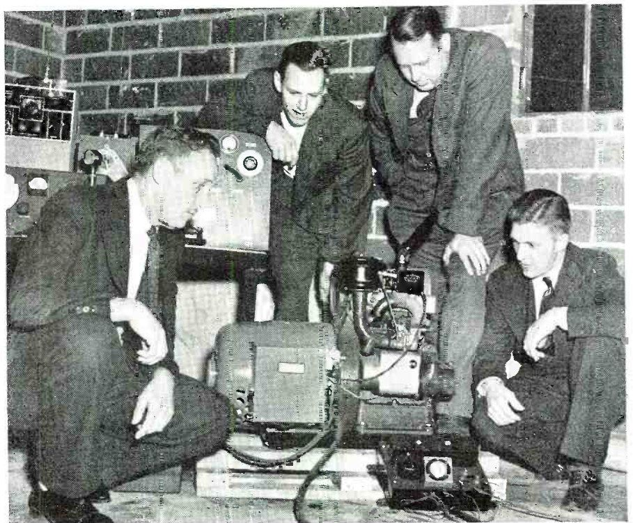
Radio amateurs examine a modern gasoline-driven generator for emergency use.
