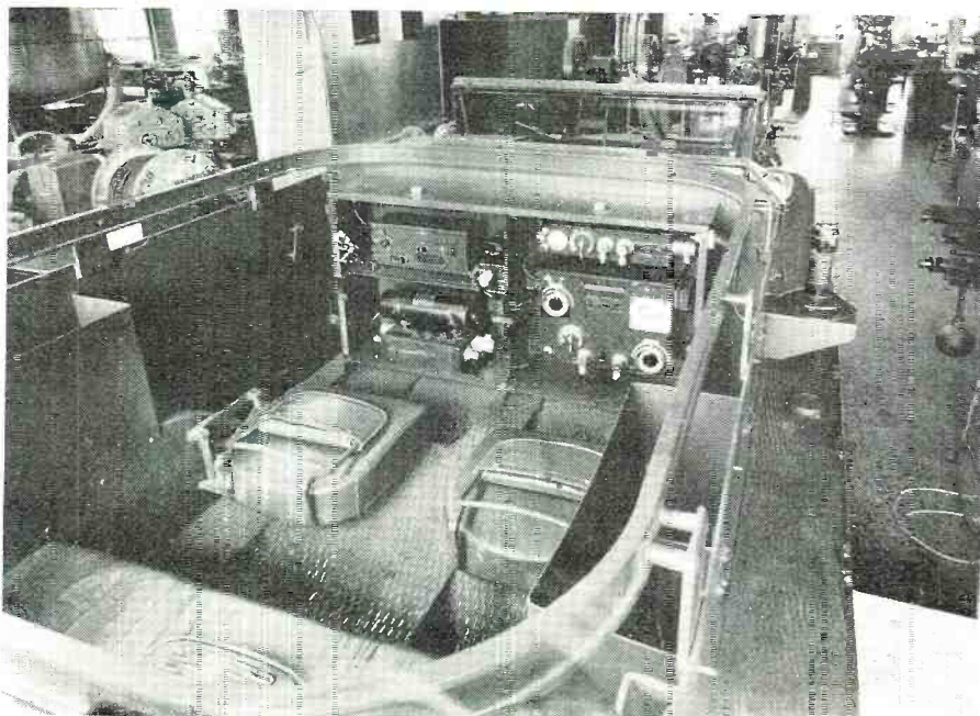
A vehicular radio set being installed in a scout car in the shop.
