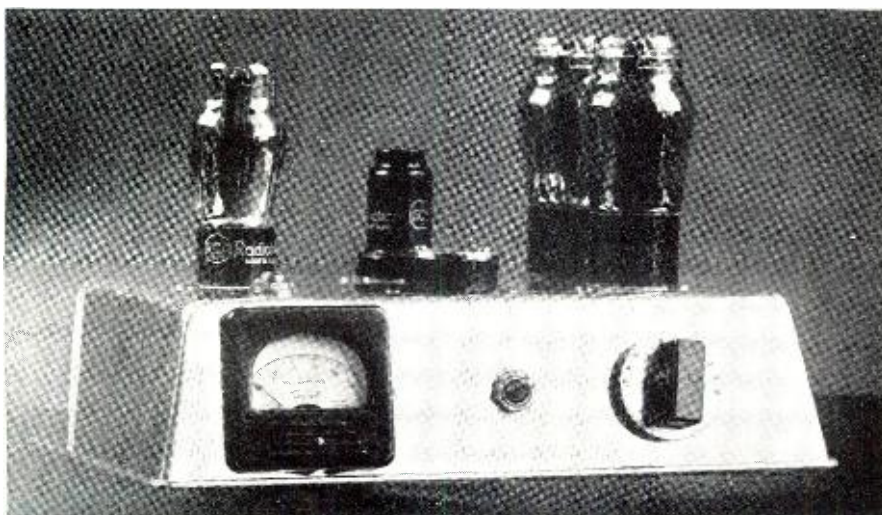
The "Blitz-4," 10-watt AC-DC Transmitter built on a tin-pan chassis.
