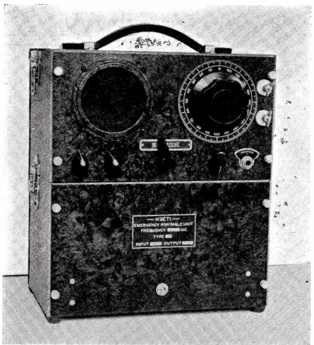
The "High-power Baby" using an HY75 transmitting tube in the receiving position with considerable success. It is AC powered.
