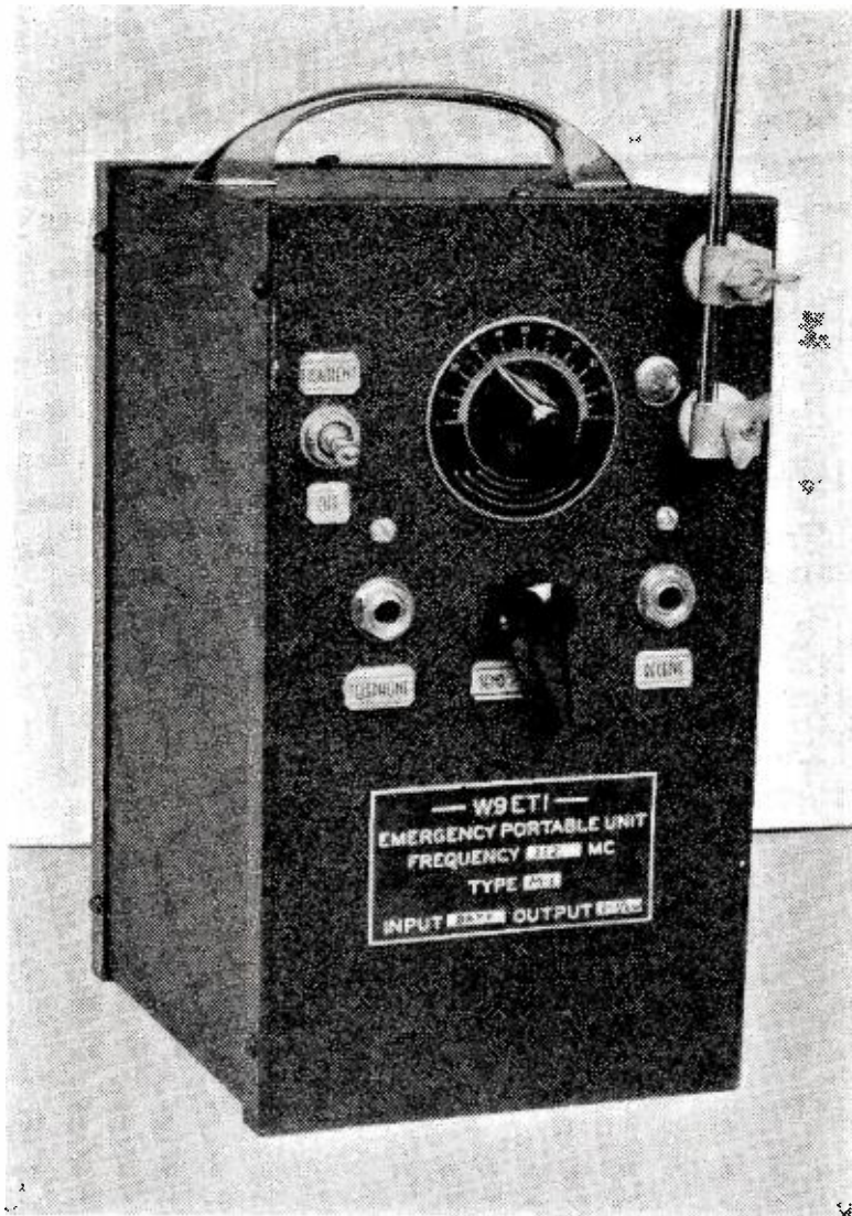
The "Beer Mug" which uses an acorn tube in the transmitting position. It did 38 miles dx.
