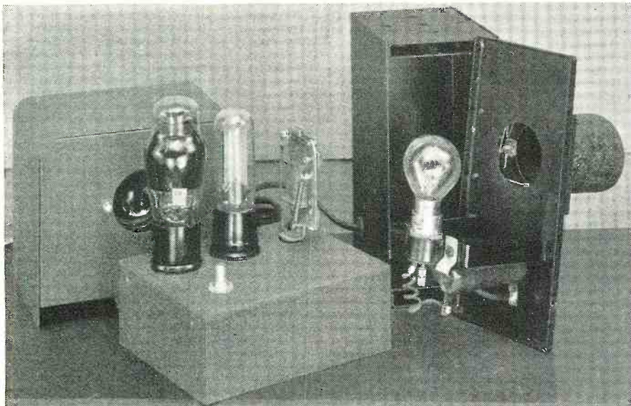
The "works" of the ham-saver photo-cell. The gadget next to the photo-cell tube is a sensitive relay which is the unit's heart.
