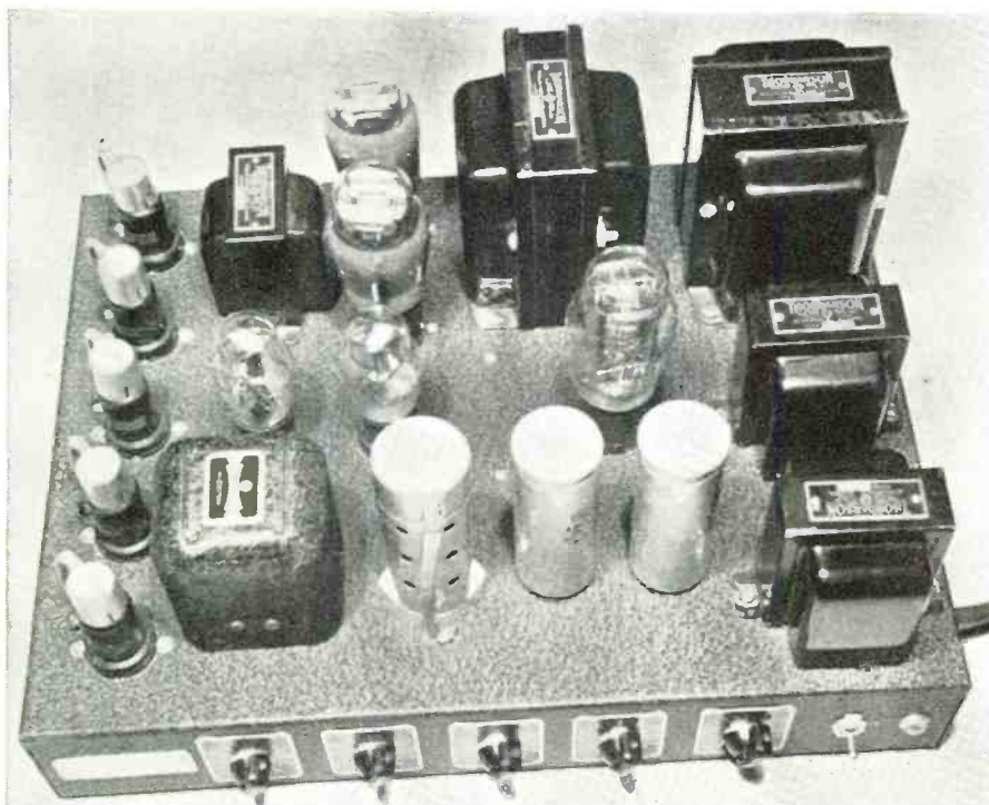
The placement of the parts permits easy servicing when it shall become necessary. No feed-back was experienced.
