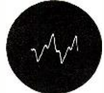
329.6 cycles or middle E, produced by silver flute. Practically a pure wave form.
