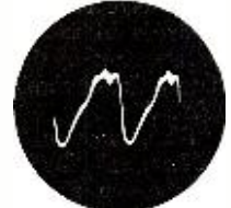
392 cycle or middle G, sounded by a soft tone on a bugle. Minimum harmonics.
