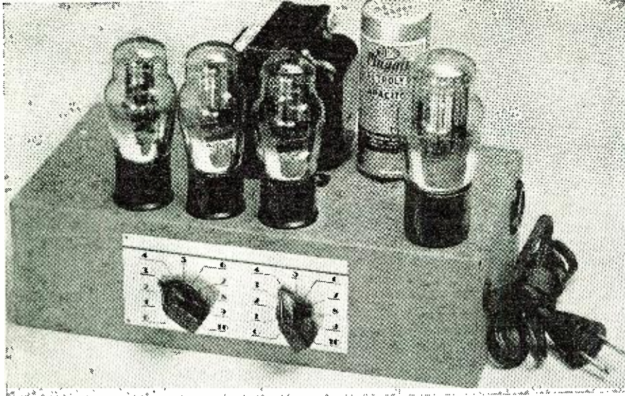
The VOX System is simplicity itself. While the laboratory model is mounted on a separate chassis, there is no reason why this unit cannot be built into the xmtr.
