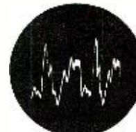
392 cycles, middle G, produced by single reed of an accordion. Note many harmonics.
