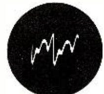
329.6 cycles as produced by a C melody saxophone. This instrument combines vibrating reed; tuned resonant chamber.
