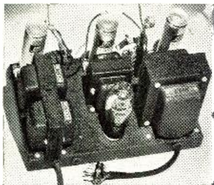
The power supply chassis connects by cable.
