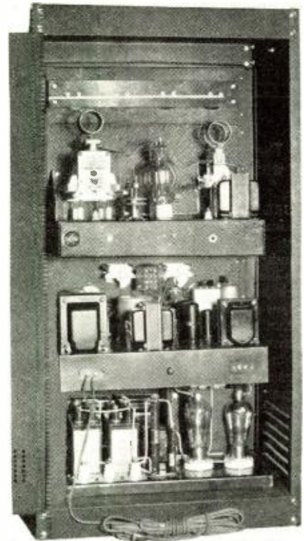
Rear view of the completed low-level modulated 150 watt-peak 600 watt transmitter.
