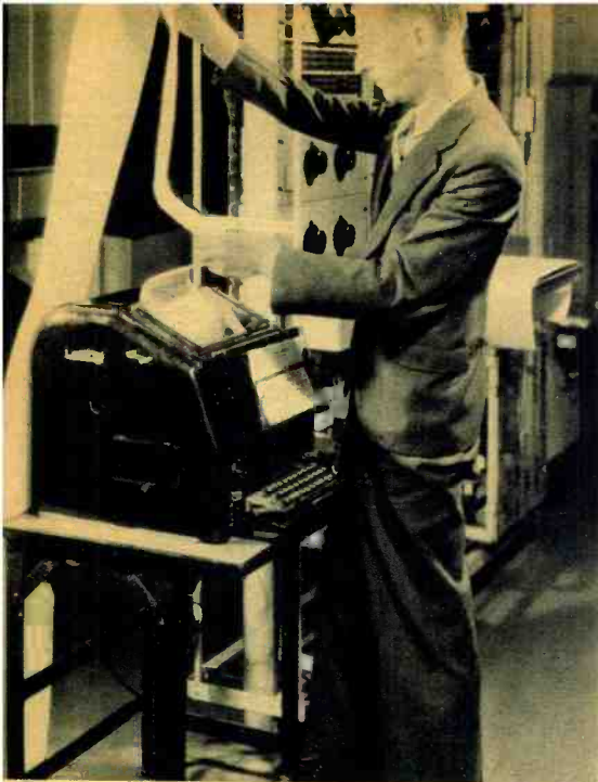
The program order for one day sent to all telephone company offices from New York. It carries all network information for all services and is sent by teletype.
