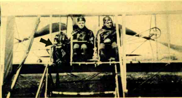
An experimental airplane wireless installation of 1912. The officers are Lt. Follett Bradley (now Colonel, Air Corps) and Lt. Henry H. Arnold (now Brigadier-General and Assist. Chief of the Air Corps).
