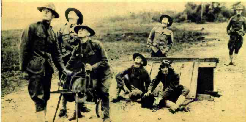
One of the early experimental "wireless" telephone ground units for contact between airplanes in flight and ground stations. Note the hand-driven generator and the ancient earphone caps.
