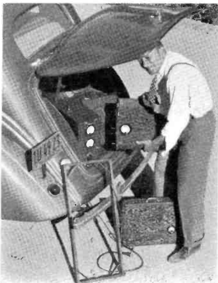
The metalloscope is so rugged in construction and so compact that it may be packed in the luggage compartment of a car and carried about.
