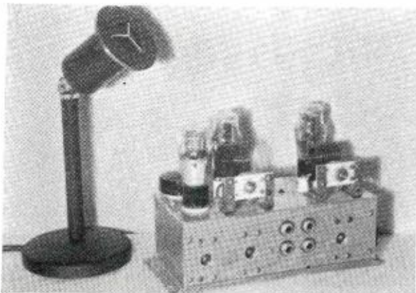
The Radio Frequency section of the miniature transmitter. It is considerably smaller than the "Salt Shaker" mike.
