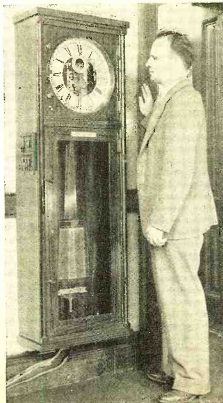
THE TRANSMITTING CLOCK This is the apparatus that sends out the familiar "peep, peep, peep" of the radio time signals
