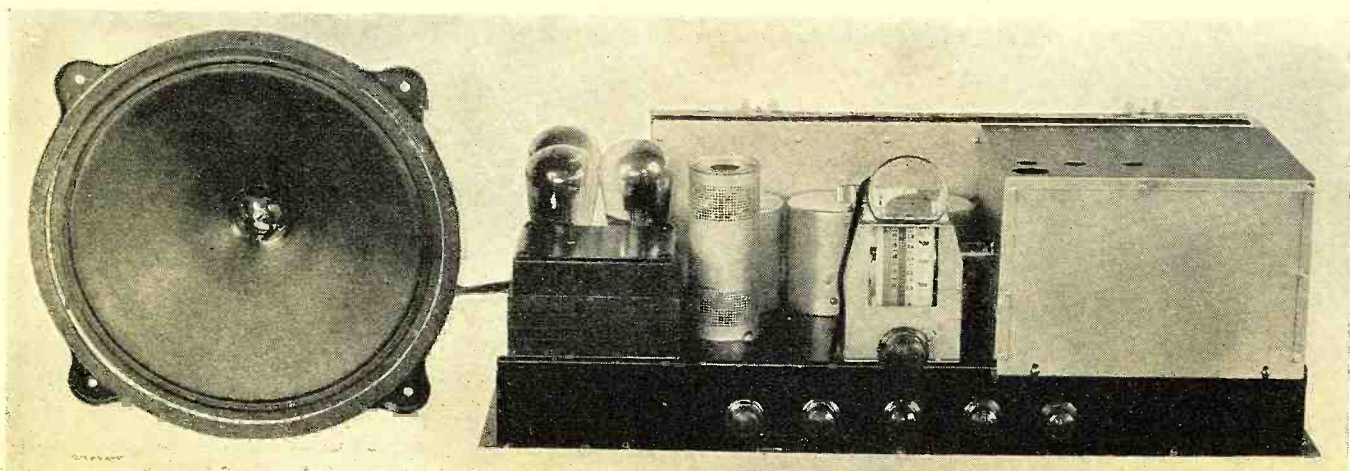
Figure 1. Complete shielding is provided. The dial is accurately calibrated in kilocycles for each of the four bands and a visual resonance meter is shown over the dial
