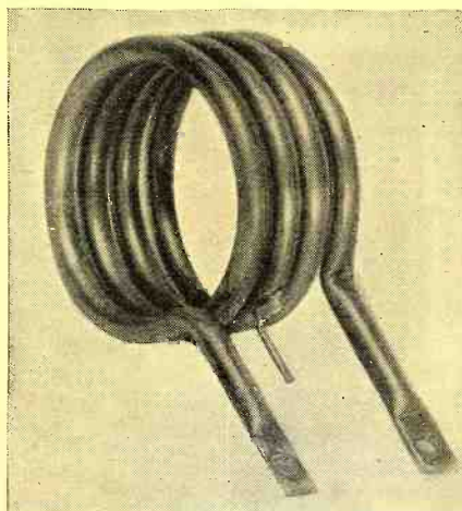
Figure 9. This is the tapped four turn low C coil used in the original experiments
