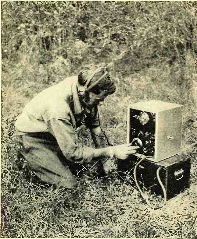
Figure 3. This semi-portable radiophone can be carried by motor or pack horse and set-up in a safe location near the fire to contact rangers on the fire line
