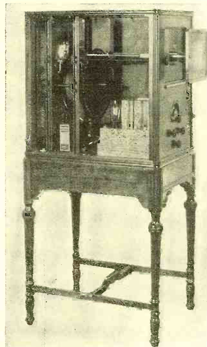
PROJECTION TELEVISOR In this new Jenkins receiver which employs the lens scanning disc, the received pictures are projected on a ground glass section which enables everyone in the room to view the living objects
