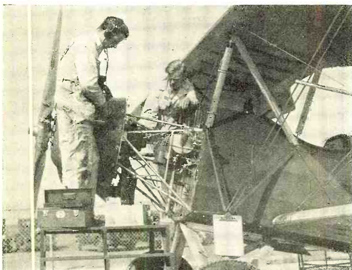
OVERHAULING IGNITION SHIELDING SYSTEM Aviation maintenance men checking the ignition shielding system of a plane so necessary for quiet operation
