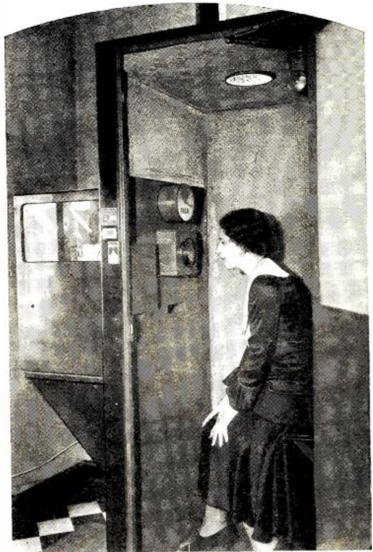
An interior view of the Vocamat booth. The illuminated dial which tells when to start talking, how long to talk and when to stop is plainly visible. The dark sector may be seen and also the hand, which had moved about 1/4 of its traverse when the picture was taken. Directly in front of the speaker is the grill box containing the microphone
