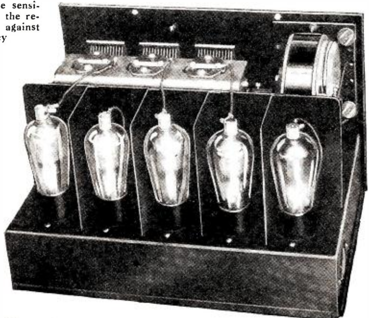
The receiver employs a total of five tubes, providing three stages of r.f., detector and pentode output stages
