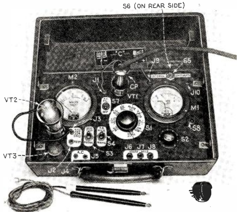
View of the tester in actual operation. Close scrutiny shows that S1 is set for a plate voltage reading, S2 for scale 8 and meter M1 reads 3.8. Reference to the chart, Figure 1, shows that the plate voltage of the tube under test is therefore 190
