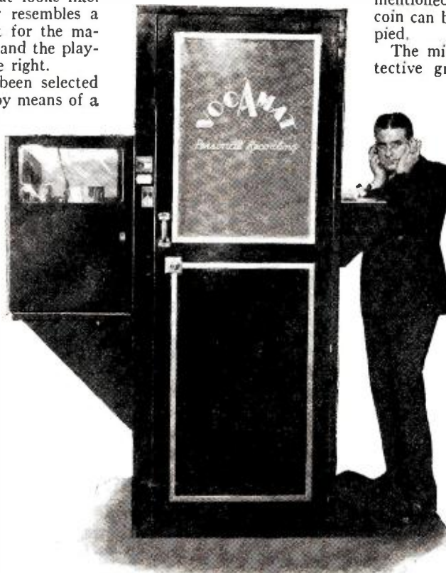
A view of the Vocamat, showing the machinery cabinet at the left and the phonograph turntable for playing back records at the right of the booth
