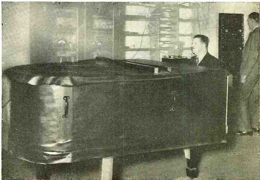
L. M. Cockaday, Editor of RADIO NEWS, playing what is probably the world's only sound-proof piano, constructed so that all the sound of the piano could be picked up by a microphone inside the case for electrical study or loud speaker reproduction
