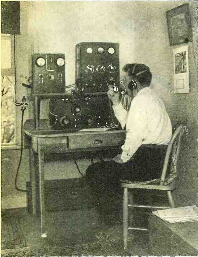
It was in amateur stations such as this that broadcasting of music started in 1919. The photo shows the vacuum tube transmitter equipment used by William Andrew Mackay at that time. The receiver shown below the transmitter is one of the first three-circuit tuners
