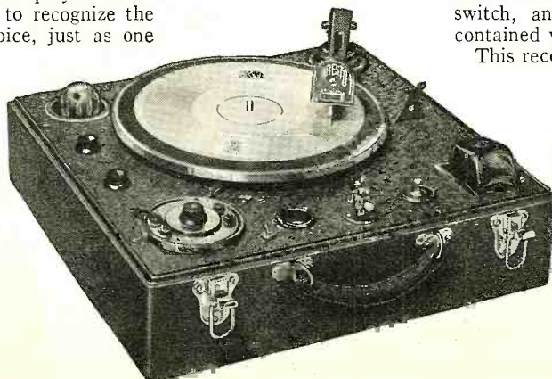
A portable unit which contains all equipment needed, in conjunction with a modern radio receiver, to record either radio programs or voice at home
