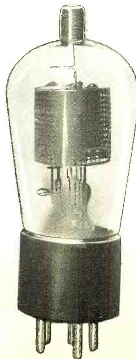
(Right) The four-element a.c. audion of today—the type of vacuum tube which makes possible the near perfection of modern receivers
