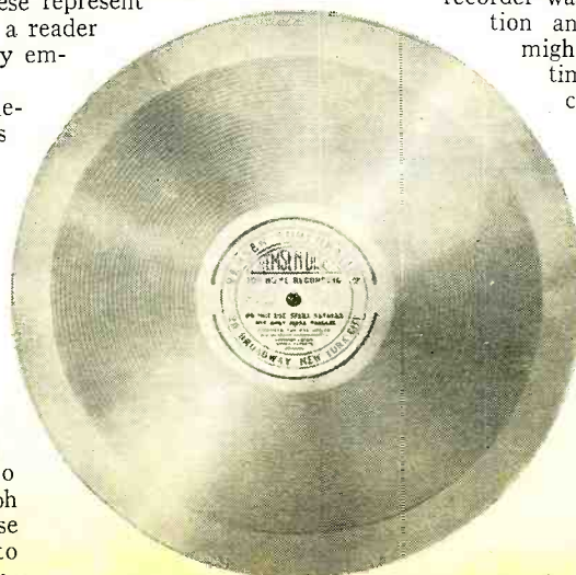
One of the recordings of a short-wave program from Chelmsford, England. The wide outside margin was left to permit date and other notations to be "dubbed in"
