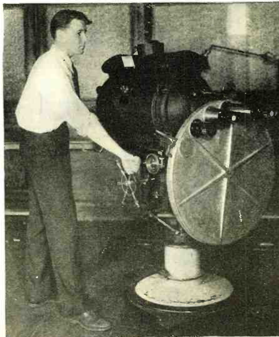
Direct pick-up television camera of the Jenkins station. Three of the possible five lenses are mounted on the scanning disc housing, the desired lens being moved into position by the handle on the outer rim of the housing. The entire camera may be moved vertically by means of the foot pedal on the base. The operator is holding the wheel which tilts the camera vertically
