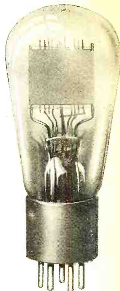
Photo and cut-away view (Figure 1, at left) of the new pentode tube. The suppressor grid is connected to the midpoint of the filament, within the tube, and therefore no external connection is required for this added element
