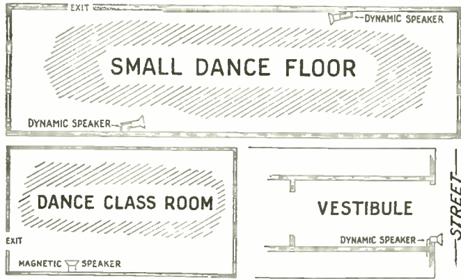
Fig. 4—Floor plan of two of the three halls constituting the Remy Dancing School, including the street entrance, where a dynamic speaker is mounted for publicity purposes
