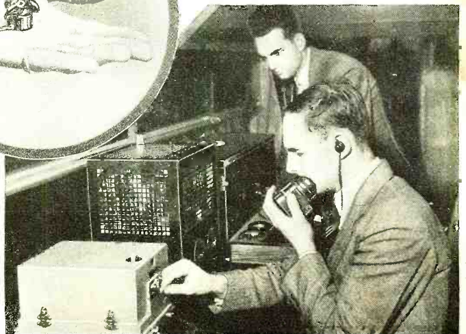
Engineers at the small one-control five-tube screen-grid receiver, on the right of which is the fifty-watt radio telephone transmitter. Both can be operated by remote control. The operator in the foreground may be seen wearing the midget headphone
