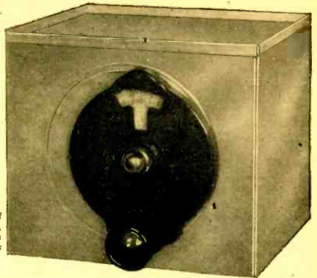
A shield can, of the type most used in present-day receiver construction, makes a handy metal cabinet for a plug-in wavemeter; for it keeps down the annoyance of hand-capacity.
