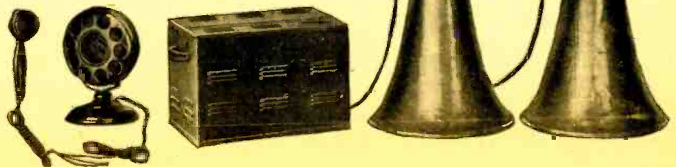
Fig. D A highly-portable Silver-Marshall amplifier with two of its speakers and microphones. One system of this type is described above.
