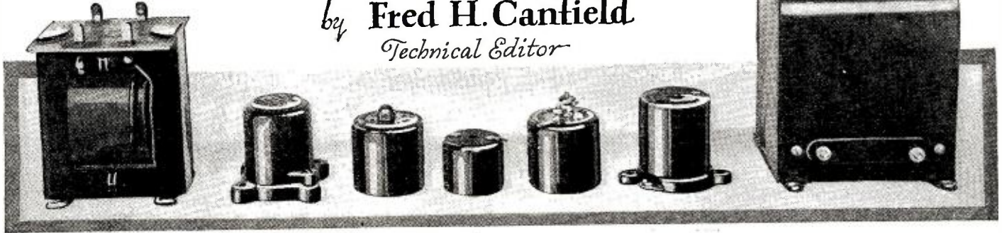
The two large cases contain chokes for use in audio-frequency filters, and the five small ones radio-frequency chokes.
