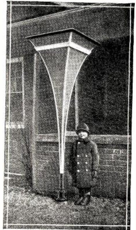
The extension of the exponential horn is the part above the white band near the top; its construction is described here.
