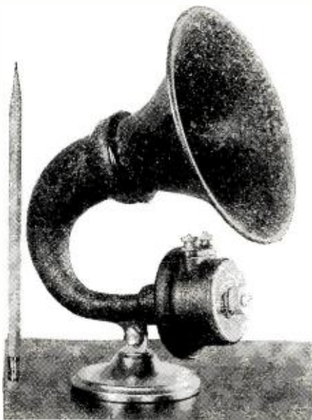
This horn is of a type recently popular. Its "cut-off frequency" is very high, because of its shortness; yet music gets through, even though it does not go so far as if the horn were longer.
