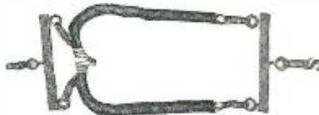
An easily installed spring aerial, useful to fans living in apartment-house districts. Photo by courtesy of Mack Co., Inc.
