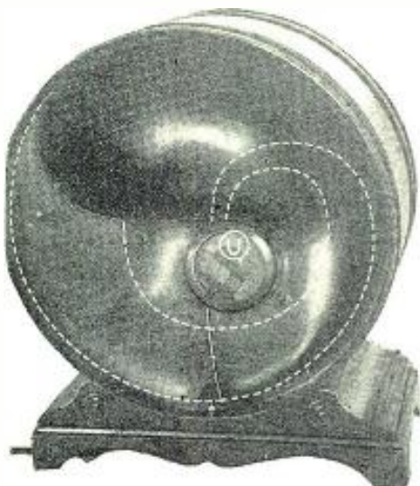
Dotted lines indicate shape of the horn which is housed inside the drum. U is the speaker unit.
