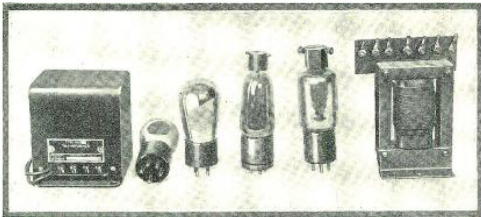
Another solution of the "electrification" problem is the use of the new A.C. tubes, which employ alternating current for their filaments. These tubes require merely a small step-down transformer, and involve but few changes in the wiring of a set. Several typical A.C. tubes and two lighting transformers are shown above. A regular "B" supply device must be used with these tubes.
