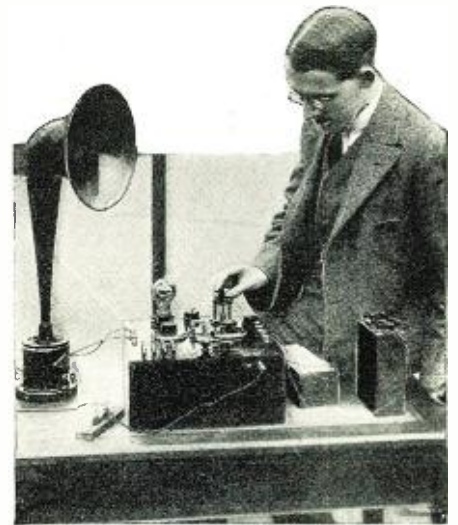
This shows the interesting crystal-and-tube combination set diagramed in Fig. 2. The change-over switches will be seen.
