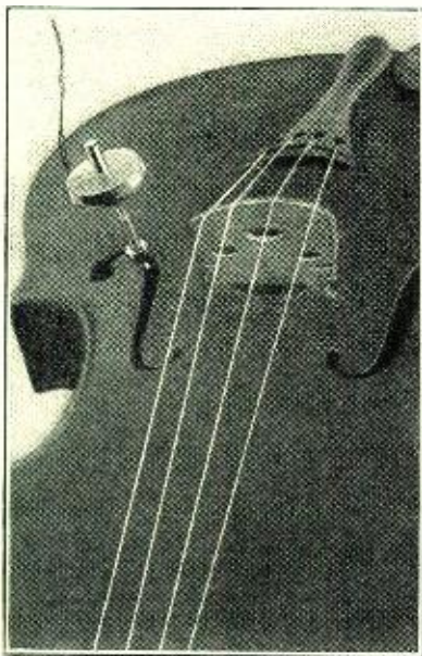
Showing detail of mounting in f-hole of violin, which does not mar instrument. With some stringed instruments it may be desirable to drill a small hole to accommodate the screw to which the microphone reed is soldered.
