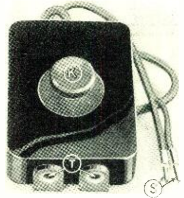
The tone control. K is the adjusting knob. The tips S go to the output of the set, while the tip jacks T take the loud-speaker cord.
