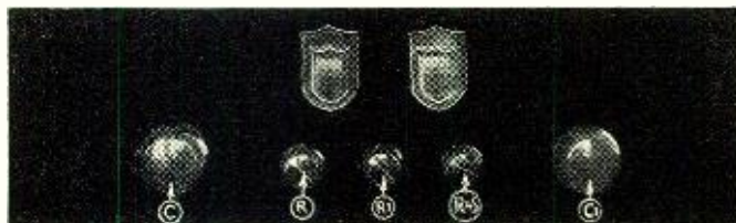
A panel view of the nine-in-line superheterodyne receiver. C and C1 are the variable condenser controls; R and R1 are the rheostats, and R4-S is the combination volume control and filament switch.
