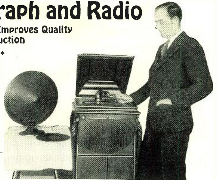
The author, illustrating the use of the "pick-up" device, proves that it is as simple to operate as the average phonograph, with the single exception that a filament switch must be closed.
