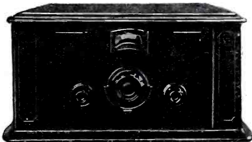
Front view of the single-control 6-tube receiver. The tuning knob is the large one in the center of the panel. Photos courtesy The Magnavox Company
