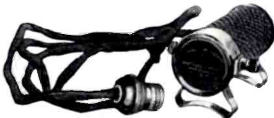
Fig. 6. A direct-current trickle charger which will deliver three-tenths 0.3 of an ampere to any six-volt storage battery. Incidentally, it can also be used for charging storage "B" batteries.
