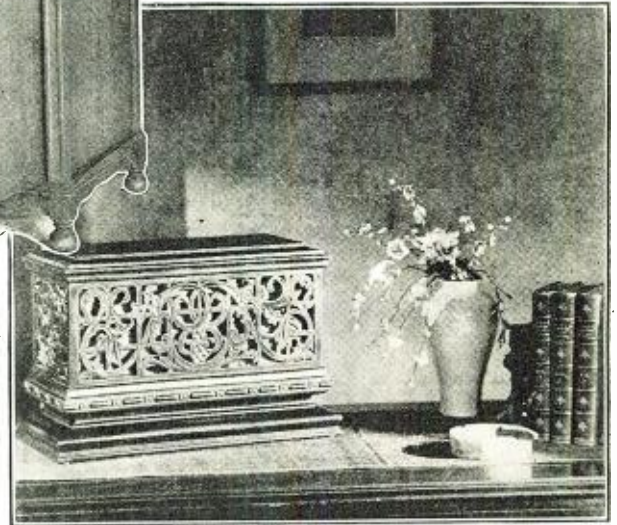
Fig. 3. Two striking examples of the advancements made in the horn-type loud speaker. The speaker above contains a compact horn with a total length of 7 feet and is capable of reproducing, with marked fidelity, the low notes usually lost in other speakers. The speaker is equipped with a large Baldwin unit.
