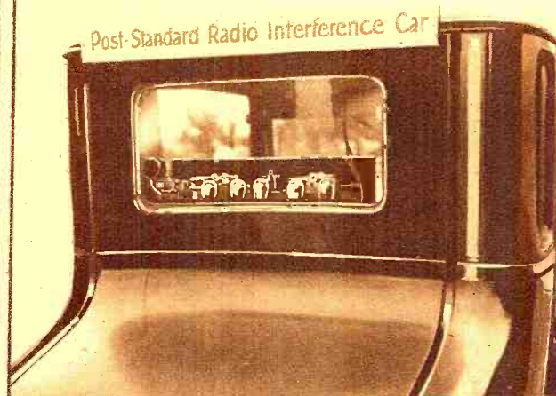
Sources of radio interference in Syracuse, N. Y., are investigated with the aid of this car, supplied by a newspaper of the city, which patrols the streets every evening. The loop shown in the view at the left is used to detect the source of any alternating-current hum, which is tracked down at once by an experienced lineman. © Syracuse Post-Standard.
