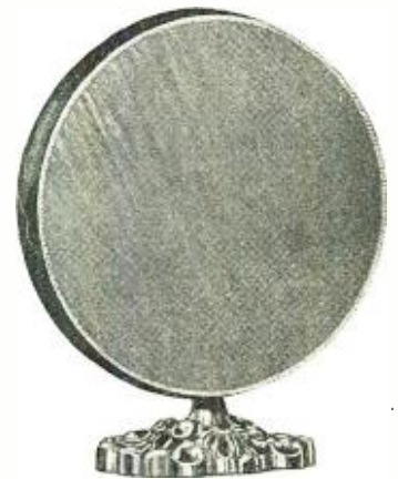
A typical form of disc speaker with characteristics somewhat similar to a fixed-edge cone speaker.
