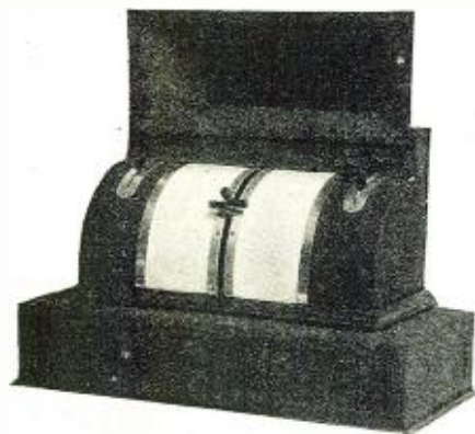
Instead of tuning with the usual dials, this receiver's condensers are adjusted by levers. Photo by courtesy of Duinn Mfg. Co.
