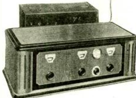
Behind the five-tube receiver may be seen the eliminator which supplies all the necessary power for it.
