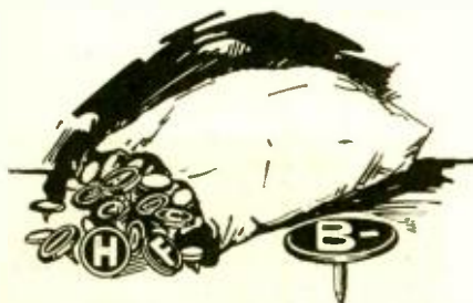
Fig. 3. On the head of the push-pins, shown in the above sketch, are engraved the different symbols, which may mark the terminals on a set.
