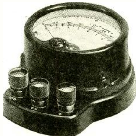
Fig. 4. A portable double-range voltmeter for testing all types of "A," "B" and "C" batteries, or other direct-current voltage sources. There is one negative binding post and two positive binding posts, low- and high-voltage.
