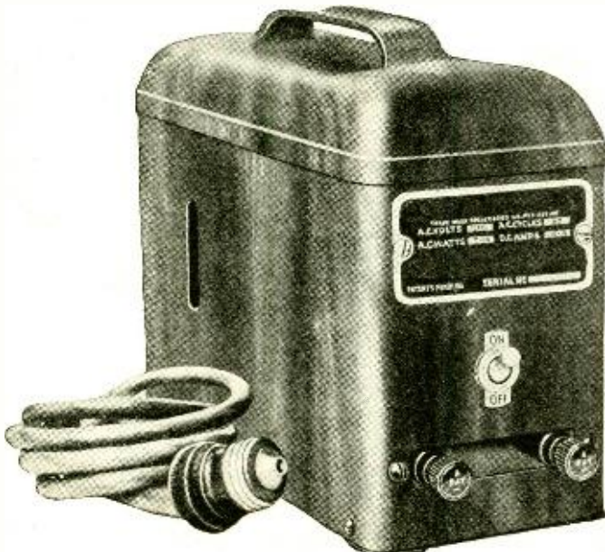
Fig. 15. (Left) An "A"-battery trickle-charger for use on A.C. lines. It employs an electrolytic rectifier. Three charging rates are obtainable, controlled by a switch inside the case. The charger is turned on and off by the toggle switch on the front of the case. It is possible to operate the receiving set while the charger is on.
