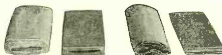
Fig. 7. At the left is shown the appearance of a 2- \mu f. condenser before and after the paraffin impregnation. The other two windings are for 1- \mu f. condensers.
