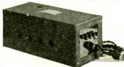
Receivers using plate voltage up to 135 volts can be supplied with the necessary power from this eliminator.
