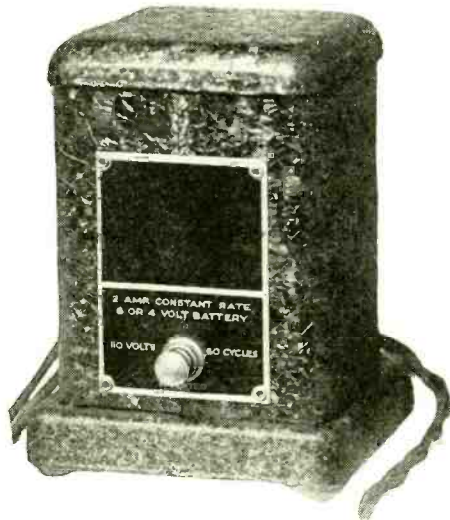
Fig. 8. A console-model storage-"A"-battery charger with a 2-ampere rate, sufficient for most purposes. It employs a very efficient form of mechanical rectifier.
