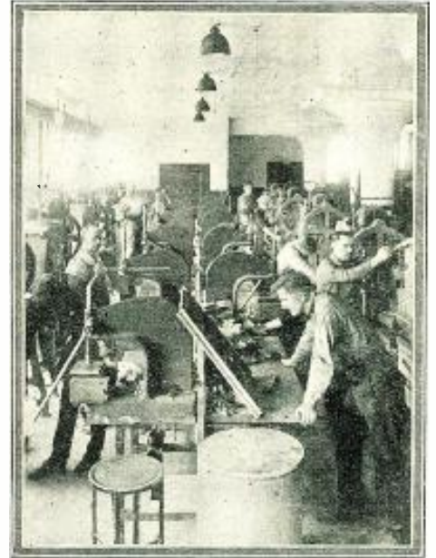
The molding department makes the different insulating composition parts, using thermostatically-controlled presses. Courtesy of A. H. Grebe & Co., Inc.
