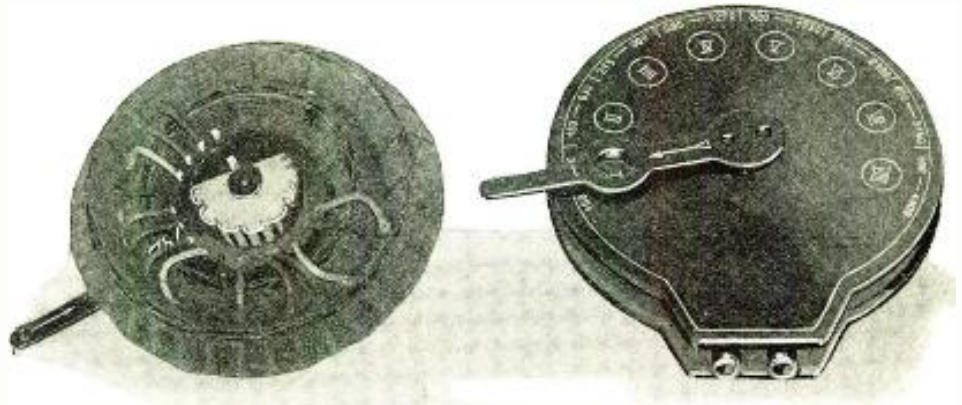
In the left view the cover of the inductance has been removed to show the type of winding. The wave bands covered are indicated at the various points in the right hand view. Courtesy of Ideal Radiotelefon & Apparatefabrik.
