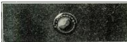
The Family Receiver has one control on the panel, which switches on the filaments and tunes the set.
