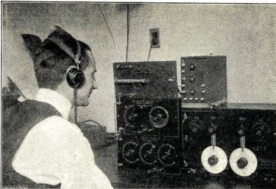
A multiplex receiving system that can pick up signals from five different stations at the same time on a single aerial.
