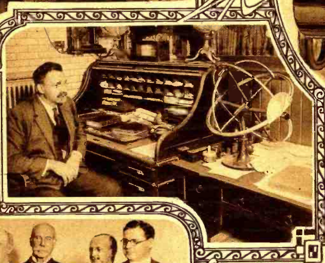
Left: Captain Robert Huntington, Principal of the Navigation School at Seamen's Church Institute, has done more for the sailor ill at sea than any other man in the world. He conceived the idea of prescribing treatment by radio for sick seamen on vessels carrying no doctor. At the right is a spherical angle calculator for locating a vessel's position, a time-saving device invented by the captain. ©Gilliams Service, N. Y.
