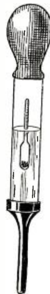
Fig. 8. A hydrometer used for determining the specific gravity of the electrolyte of a lead plate storage battery.
