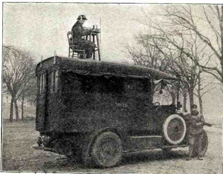
Fig. 7. The two meter set was installed on top of a car to determine the effect of obstacles upon the propagation and also the range over which it was possible to work.
