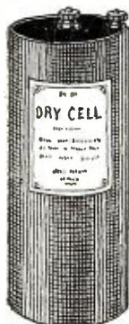
Fig. 1. A standard type of No. 6 dry cell which develops a pressure of 1½ volts.
