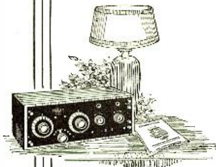
The justly famous Crosley Model VI, a two tube set incorporating one stage of tuned radio frequency amplification and detector. Price—$28.00.
