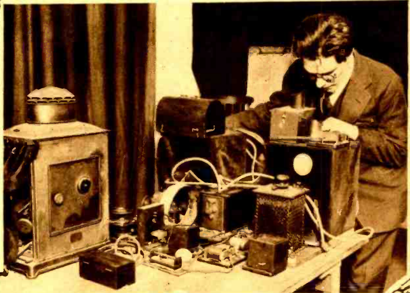
Upper Right Photo Shows Captain A. J. Hillary, Master of the Mail Boat "President," Receiving Information By Radio as to the Number of Bags of Mail on Board an Incoming Liner. Above: A Picture of a One-Kilowatt Ship Type of Quenched Spark Transmitter. This is the Most Efficient Form of Spark Transmitter, But, Due to the Greater Efficiency of C.W., They Are Being Converted Into the Latter. Aside From the Quenched Spark Gap, All the Other Apparatus is Made Use of in the Conversion.
