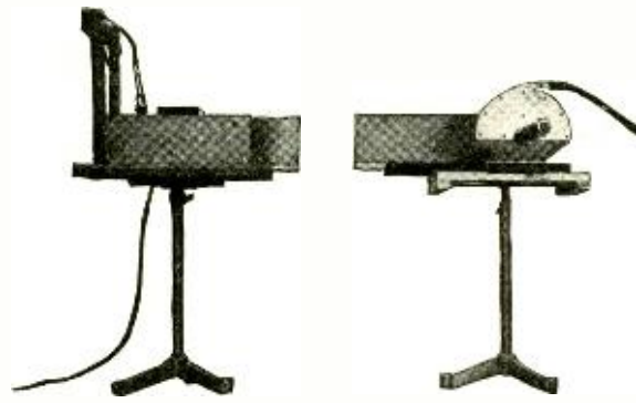
Fig. 62. General View of the Author's Apparatus For Showing Experiments With Short Electric Waves, Illustrating Their Similarity To Light Waves, and the Opacity or Transparency of Various Substances.
