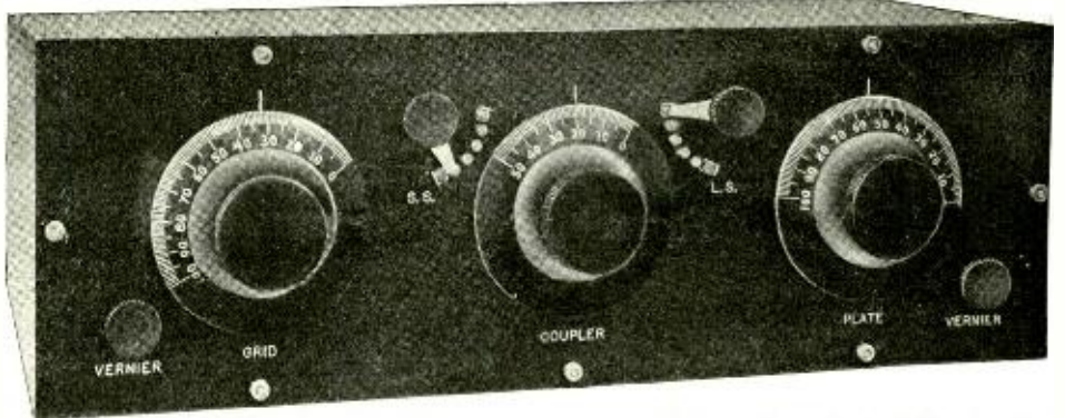
A Standard Three-Circuit Regenerative Receiver, the Circuit of Which is Shown in 2 of Fig. 12. The Controlling Knobs, from Left to Right, Are, the Grid Variometer, the Variocoupler and the Plate Variometer. Vernier Knobs, for Fine Adjustment, Are Seen in Each Corner. Primary Adjustments Are Made with the Switch-Arms S.S., L.S., and the Coupler Knob. Final Adjustments Are Made by the Simultaneous, Alternate Back-and-Forward Motion of the Grid and Plate Variometer Knobs and Possibly the Verniers.
